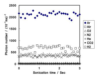
Fig. 3 Effect of dissolved gas on MBSL
