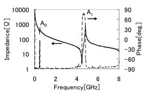
Fig. 4 Measured impedance and phase characteristics of 1-port resonator (wide range)
