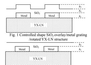
Fig. 2 Flattened-SiO<sub>2</sub> overlay/metal grating /rotated YX-LN structure
