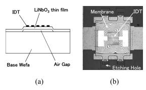
Fig. 3 Device structure (a) side view and (b) Top view
