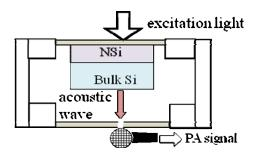
Figure 1 Arrangement of the transmission PA method.
