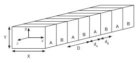
Fig. 1. Rectangular cross-section nanowire superlattice.
