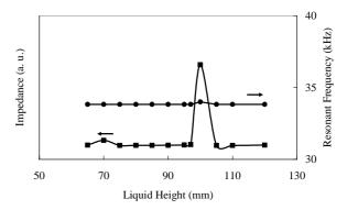
Fig. 4 Dependence of the liquid height on calculated resonant frequency and impedance of the BLT transducer driving at 34 kHz.
