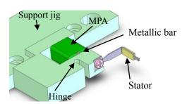
Fig.3 Construction of an L-shaped ultrasonic actuator with preload control MPA.
