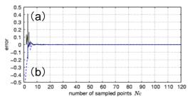
Fig. 1: Error  $\varepsilon(\theta_s)$  between the interpolated peaks and the true peaks of correlation functions between simulated sinusoidal functions (a)  $P_0$ =1, (b)  $P_0$ =-1.
