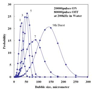
Fig. 1 The development of the bubble size distribution by the sequential burst of ultrasound.
