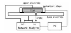
Fig. 1 Probe system to pick up induced charge
