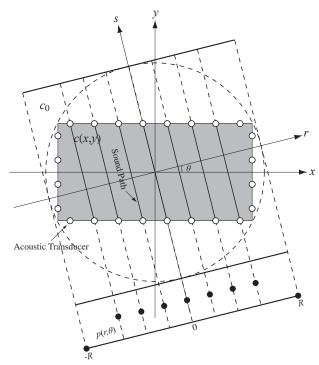
Fig. 1 Principle of A-CT in rectangular space.
