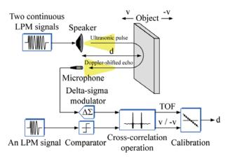
Figure 1: Design of the proposed method of accurate distance measurement
