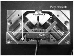
Fig.1 New design for minimization of V-shape motor.
