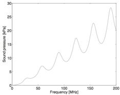
Fig. 2 Frequency characteristics for sound pressure of the water loaded polyurea ultrasonic transducer.
