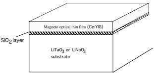
Fig. 1 Configuration of the MO film on LT or LN substrates.
