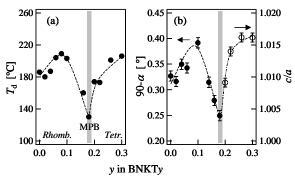
Fig. 3 Compositional dependence of (a) depolarization temperature,  $T_d$ , and (b) rhombohedral distortion, 90°- $\alpha$ , and tetragonality, c/a, for BNKTx.
