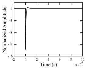
**Fig.7** Simulation of impulse response of loudspeaker based on the system.
