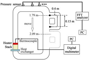
Fig. 1 Diagram of measurement system.
