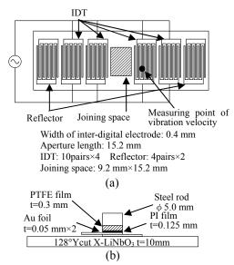
Fig.1. Schematic diagram of construction of SAW joining system. (a) Top view and (b) Side view (t: thickness  $\phi$ : diameter)
