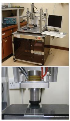
Fig. 1. The in-house automated equipment model for the ultrasonic thin-die bonding (top) and the zoom-in view of the 40 kHz, 500 W piezoelectric ultrasonic transducer (bottom).
