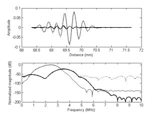
Fig. 3 Comparison of the pulse-echo line from the NPS (dotted) with the linear plus quadratic output from the SVF model (solid).
