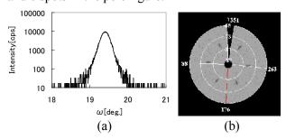
Fig. 2 (a) Measured rocking curve and (b) pole figure of thin LiNbO3 film with X-Ray Deffraction
