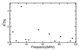
Fig.2 Analytical result of  $K^2$  in each mode for lamb wave.
