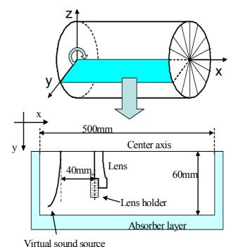
Fig.2 Calculation model for FDTD simulation
