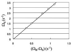
Fig.1 Relation between  $(\Omega_B-\Omega_S)$  giving the applied torque and  $\Omega_S$  representing the shear rate.
