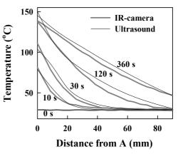
Fig. 4 Surface temperature distribution of the steel plate and its variation during heating.
