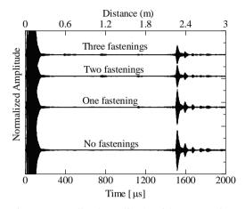
Fig. 5 Normalized amplitude with propagation time for different fastenings.
