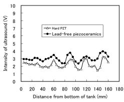
Fig.4. Variation of the intensity of ultrasound of the cleaner with distance from the bottom.
