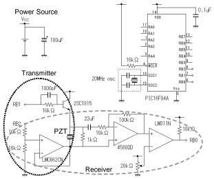
Fig. 2 Transmitter and Receiver Circuit.
