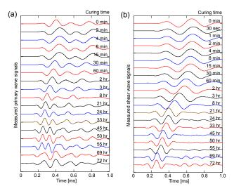
Fig. 4 Evolution of measured signals for sf=0.6 at fixed vertical stress  $\sigma'_v$ =21kPa: (a) Primary wave; (b) Shear wave.
