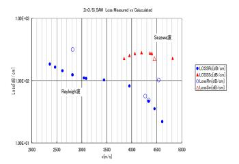
Fig. 4 Calculation result of loss vs velocity.
