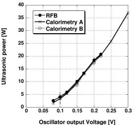
Fig. 4 Measured ultrasonic power by RFB and calorimetry at 1 MHz without multi-reflection.
