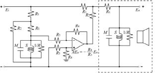
**Fig.6** System for improvement of impulse response of loudspeaker.
