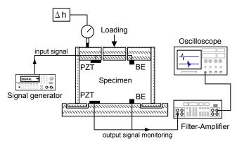
Fig. 2 Experimental setup. BE and PZT denote a bender element and piezo-disk element, respectively
