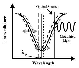
Fig.1. Principle of LPG vibration sensor.
