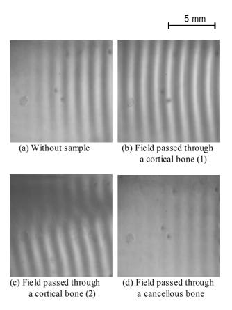
Fig. 2 Schlieren images of ultrasonic fields at 1.03 MHz.
