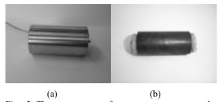
Fig. 5 The appearance of a prototype motor and assembled SMC core (a): Motor Ass'y, (b): Core Ass'y
