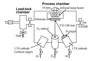
Fig. 1 Configuration of RF-magnetron sputtering system.
