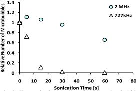
Sonication Time [s] Fig.6: Change in the number of  $10~\mu m$  microbubbles as a function of sonication time at a power of 40~W.
