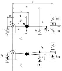
Fig. 1 Lumped parameter model of a hinged magnetic relay, (a) free state, (b) make state
