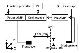
Fig.2 Lens Performance Measurement System
