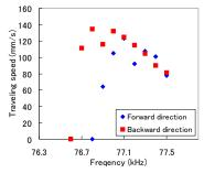
Fig.4 Traveling speed vs frequency characteristic (No Load、at 90Vrms input)
