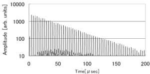
Fig. 1 Multiple roundtrip (60turns) of SAW on a quartz ball SAW device
