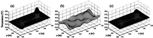
**Fig. 2** Exact and reconstructed temperature distributions. (a) Exact distribution. (b) Reconstructed from projection data of 45 ° equal angular intervals. (c) Reconstructed by the proposed method.
