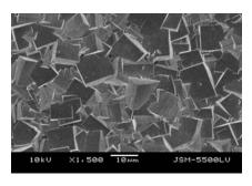
The SEM image of hydrothermally synthesized PZT polycrystalline film on Ti substrate of bimorph type vibrator
