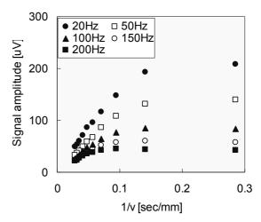
**Figure3.** Inverse of linear flow rate (v) dependence of signal amplitude (chopping frequency=20-200Hz)
