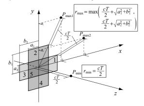
Fig. 2 Calculation range of the distance |r|.
