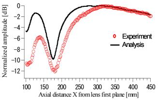
Fig. 3 On-axis sound pressure
