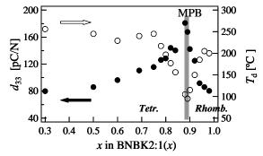
Fig. 4 The piezoelectric constant,  $d_{33}$ , and depolarization temperature,  $T_d$ , of BNBK2:1(x).
