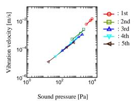
Fig. 4 Relationship between sound pressure and vibration velocity of sample MS1000 at the converging point.
