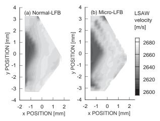
Fig. 4. LSAW velocity distributions measured for Z-cut ZnO single crystal specimen.
