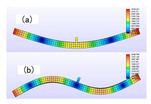
Fig. 2 The first and second bending vibration modes of plate shaped vibrator Valid amplitude ratios are, (a):1800/3036=0.59;
