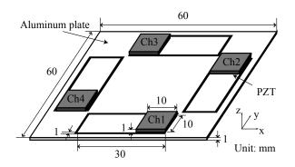
Fig. 2 Proposed self-running ultrasonically levitated 2D stage.
