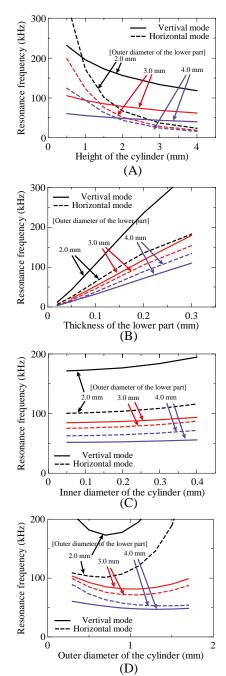
Fig. 4 Resonance frequencies against each four parameters with change of the outer diameter of the lower part.
