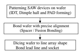
Fig. 3 Fabrication process steps
