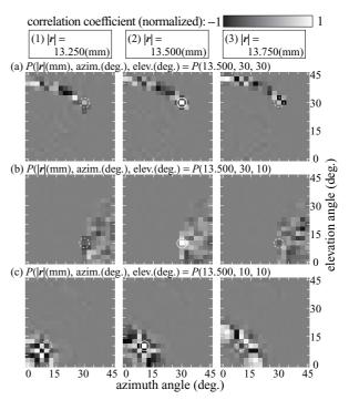
Fig. 4 Calculation results of cross-correlation coefficients: calculated using single rectangular sound source.
