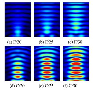
Fig.1 Calculated sound pressure distribution. F: Flat reflector, C: Concaved reflector, /20, /25, /30: Sound source diameter [mm].
