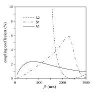
Fig.5 Coupling coefficient for free surface calculated by the acoustic velocity difference method.
