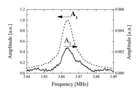
Fig. 2 Resonant spectra for the fundamental and the second-harmonic components.
