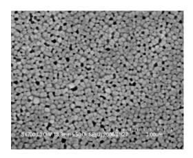
Fig. 2 SEM image of etched surface of ZnO film.
