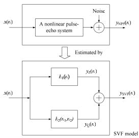
Fig. 1 Identification of a nonlinear pulse-echo system (NPS) using a SVF model.
