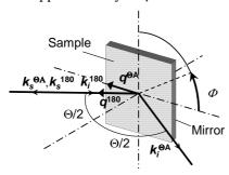
Fig. 2 RI $\Theta$ A scattering geometry where  $\Phi$  is the in-plane rotation angle.
