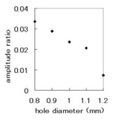
Fig. 3 Effect of hole diameter on point spread function
