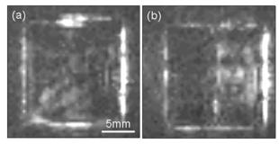
Fig.3 ASEM image of an iron foil: Original sample (a) and one after folded (b).
