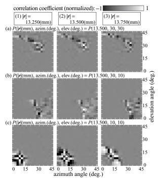
Fig. 3 Calculation results of cross-correlation coefficients: calculated using five-element rectangular array sound source.
