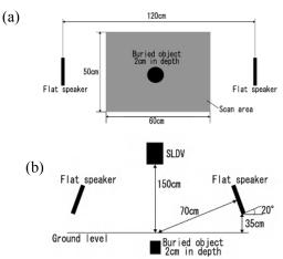
Fig.4 Experimental set up for outdoor experiment (a) Upper view (b) Side view
