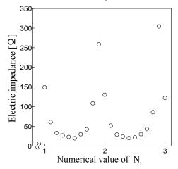
Fig.4 Relationship between numerical value of  $N_i$  and electric impedance.
