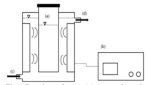
**Fig. 1** Experimental set up (a) reactor, (b) sonicator, (c) cooling water inlet, (d) cooling water outlet
