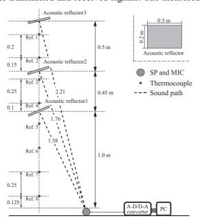
**Fig. 2** Experimental setup. Vertical temperature distribution was measured by three sound probes.
