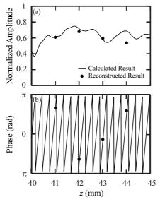
Fig. 3 Reconstructed and calculated sound field on z-axis.
