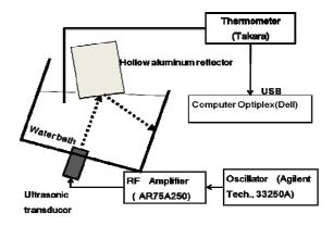
Fig. 1 Schematic diagram of the calorimetric measurement system.
