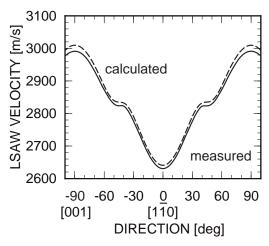
Fig. 3. Angular dependences of LSAW velocities measured for (110)Ge standard specimen using micro-LFB device.
