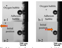
Fig.2 Interactive force between two bubbles.
