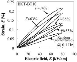
**Fig. 2** The strain behavior of BKT-BT10 ceramic under unipolar driving of electric field, *E*, from 0 to 80 kV/cm.
