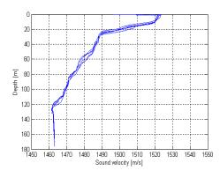
Fig. 2. Sound speed profiles derived from XBT casts over the period of 5 hours experiment.
