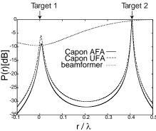
Fig. 4 The normalized brightness distribution from a pseudo echo in the case that two targets are separated by  $0.41~\lambda$ . Target distances are estimated using the beamformer method, the Capon method with UFA, and the Capon method with AFA.
