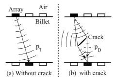
Fig.1 Transmitted wave (  $p_T$  ) and diffracted wave from a crack (  $p_D$  )
