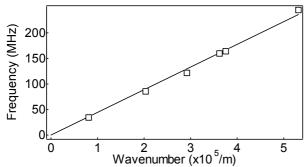
Fig. 3 Dispersion relation of acoustic phonon in PMMA obtained with the millisecond Brillouin spectroscopy over the wavenumber range from  $k = 8.1 \times 10^4$  m<sup>-1</sup> to  $k = 5.3 \times 10^5$  m<sup>-1</sup> at 300 K. The experimental points ( $\Box$ ) are well fitted by a straight line, of which the gradient yields the phase velocity, 2860 m/s for PMMA.
