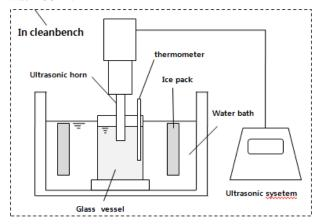
Fig. 1 Schematic of experimental set-up
