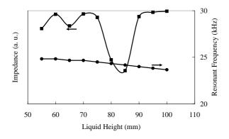
Fig. 2 Dependence of the liquid height on calculated resonant frequency and impedance of the BLT transducer driving at 25 kHz.
