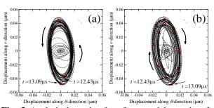
**Fig. 3** Analytical result of surface particle motion for high frequencies at (a) outer surface and (b) inner surface.
