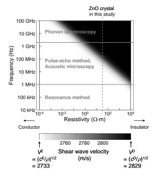
Fig. 1 Theoretically estimated resistivity and frequency dependence of the shear wave velocities of a ZnO crystal. White part and black part correspond to the  $V^{\rm E}$  and  $V^{\rm D}$  values, respectively.
