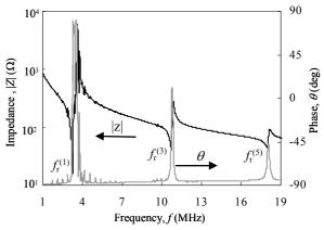
Fig. 2 Frequency dependence of impedance, Z, in the (15) mode for KN-Mn0.1 with wide frequency range.
