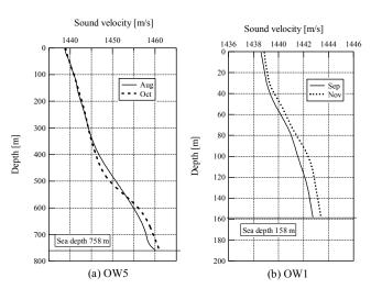
Fig. 1 Sound velocity profile of Lűtzow-Holm bay
