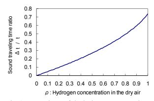
Fig. 1 Dependence of the hydrogen concentration  $\rho$  in the dry air, to the ratio of the sound traveling time in the dry air t, and traveling time difference  $\Delta t$  between the dry air and the hydrogen contained dry air according to eq. (3).
