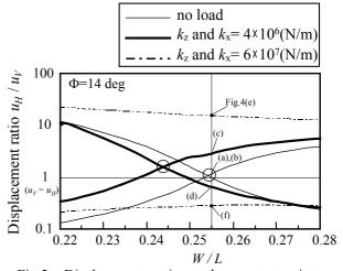
Fig.5 Displacement ratio at the contact point correlated with width-to-length ratio W/L depended on the load of springs.
