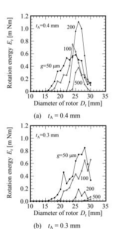
Fig. 4 Rotation energy of rotor depending on rotor diameter.
