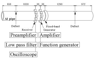
Fig. 1 Schematic illustration of experimental apparatus
