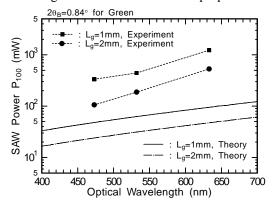
Fig. 6 SAW power  $P_{100}$  vs optical wavelength.
