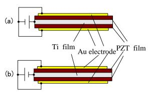
Fig.2 Polling processes for bimorph type vibrators with hydrothermally synthesized PZT polycrystalline films
