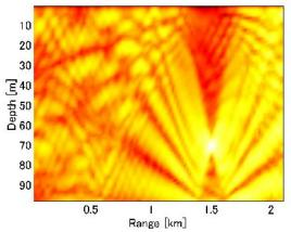
Fig. 3 TRSF for the target after traveling wave is deleted.
