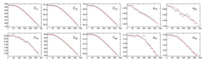
Fig. 2 Temperature dependence of elastic and piezoelectric coefficients of LiNbO<sub>3</sub>. The units are GPa for  $C_{IJ}$  and  $C/m^2$  for  $e_{IJ}$ .
