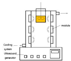
Fig. 1. Scheme of ultrasonic bath and reactor
