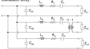
Fig. 4 Concentrated constant equivalent circuit for the disk bender transducers array having differential connections.
