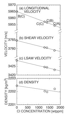
Fig. 2. Cl concentration dependences of acoustic properties of synthetic silica glass specimens.
