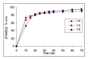
Fig.4 Effect of the molar ratio of oil to methanol on the conversion of FAMEs. Concentration of KOH was 0.7%
