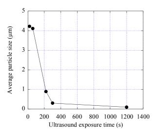
Fig. 2 Relationship between ultrasound exposure time and average particle size of nanometer-sized diamond particles
