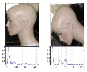
Fig.1. The face and the ultrasonic echo signal
