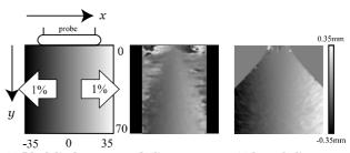
(a) Ideal displacement (b) linear scan (c) hyperbolic scan Fig. 3 A model of lateral-direction deformation and estimated displacements
