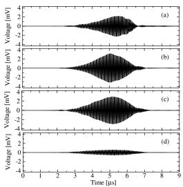
Fig. 3 : Instances of waveforms received by PVDF film with thickness of (a) 19  $\mu$ m, (b) 23.75  $\mu$ m, (c) 28  $\mu$ m and (d) 38  $\mu$ m respectively.
