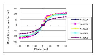
Fig 4 Input signal phase difference vs. RPM
