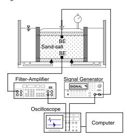
Fig. 2. Experimental setup. BE denotes a bender element.
