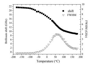
**Fig. 4** Temperature dependences of Brillouin shift and FWHM of a glycerol solution (65 mol %).
