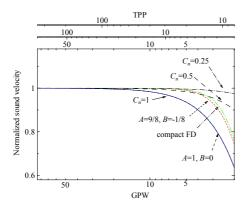
Fig.2 Numerical sound velocity v.s. GPW or TPP.
