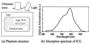
Fig.2 Phantom structure and optical property of ICG
