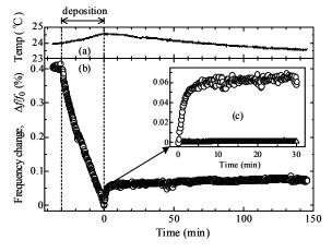
Fig. 2 Changes of (a) temperature and (b) resonance frequency of the Ag/Si specimen before, during, and after the deposition. Ag film is 255 nm thick. (c) An inset enlarges the measured resonance frequency  $(\bigcirc)$  and temperature dependence of the resonance frequency calculated from that of the elastic constants of the Si substrate  $(\triangle)$ .
