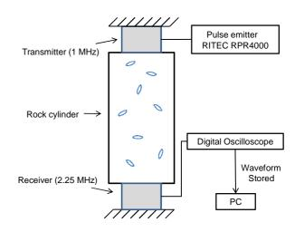
Fig. 1 Schema of the experimental setup.
