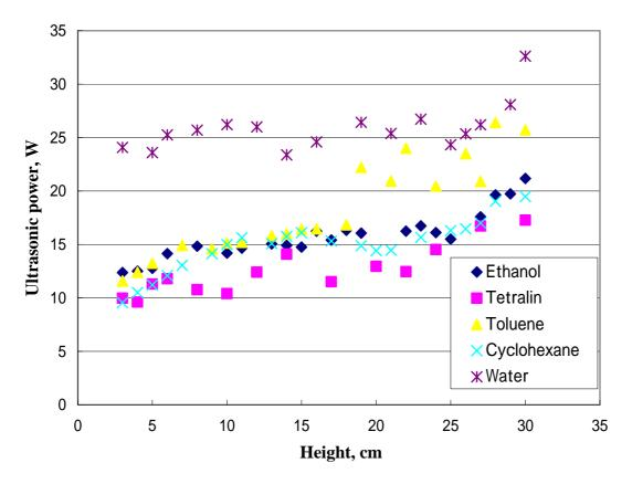
Fig. 3. Dissipated ultrasonic power as a function of the liquid height.
