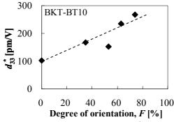
**Fig. 3** The normalized strains  $d_{33}^*$  (= $S_{\text{max}}/E_{\text{max}}$ ) of textured and nontextured BKT-BT10 ceramics as a function of the degree of orientation, F.
