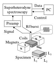
Fig. 1 Schematic representation of the measurement setup.
