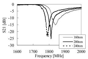
Fig. 2 Characteristics of SAW resonator of Band IV
