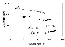
Fig.4 Shear rate dependence of viscosity obtained for aqueous solution of CTAB and Sal-Na.
