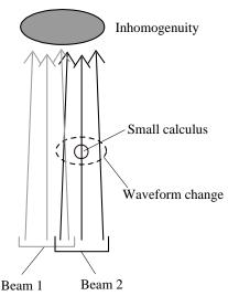
Fig. 2 Schema of the decrease of the cross-correlation value when a small calculus exists in a scan line. The waveform of an ultrasound pulse changes after passing through the calculus, and thus the cross-correlation value behind a calculus decreases.
