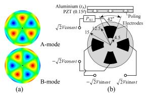
Fig. 2 Vibration patterns (a) and structure and driving condition (b) of stator.
