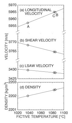
Fig. 1. Fictive temperature dependences of acoustic properties of ED-B specimens.
