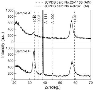
Fig. 2 XRD patterns of sample A (AlN/Silica glass substrate) and B (AlN/Al/Silica glass substrate)
