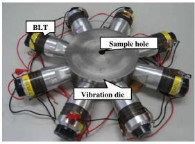
Fig. 2 the 28-kHz radial vibration system.
