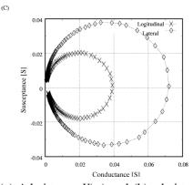
Fig. 3. (a) Admittance  $Y(\omega)$  and (b) admittance circle when the end of the tip contacted. (c) Admittance circles of chicken muscle when the end and side of the tip contacted.
