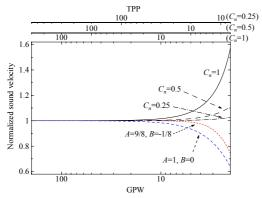
Fig. 1 Numerical sound velocity v.s. GPW or TPP.
