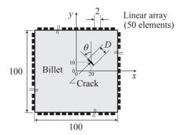
Fig.3 Simulation field of billet and internal crack
