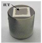
Fig.1 LN/PZT IUT onto a titanium rod.
