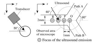
Fig.2 Schematic view of the artificial blood vessel
