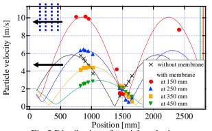
Fig.5 Distribution of particle velocity; at 400 sec. after heat supply started.
