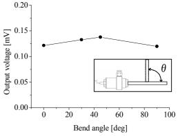
Fig. 6 Dependence on the bend angle of waveguide
