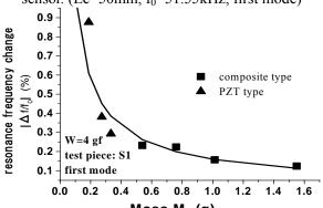
Fig.3. Experimental relationships between  $|\Delta f/f_0|$  and Mass.
