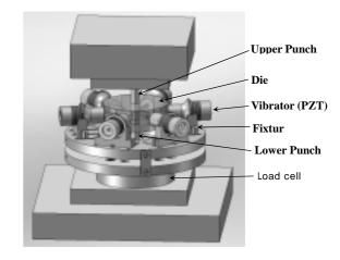
Fig. 1 The arrangement of ultrasonic vibration press
