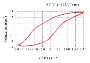
Fig.3 *P* - *E* hysteresis loops for (100)/(011)-oriented epitaxial KNbO<sub>3</sub> films grown on (100)SrRuO<sub>3</sub>//(100)SrTiO<sub>3</sub>.
