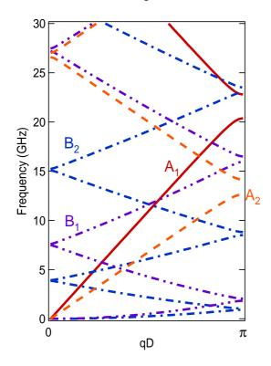
**Fig. 3.** Phonon dispersion relations of the rectangular cross-section nanowire superlattice consisting of GaAs and AlAs.
