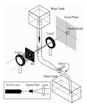
Fig.2 Experimental setup of a spectrometer and a flow system
