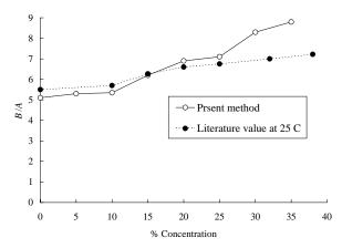
Fig.2. Measured *B/A* of aqueous hemoglobin solution.
