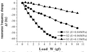
Fig.2 Characteristics of longitudinal-bar type tactile sensor. (Lc=50mm, f<sub>0</sub>=51.55kHz, first mode)
