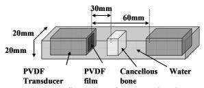
Fig.2 Configuration of an acoustic tube
