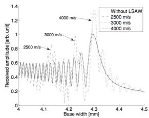
Fig. 5 V(W) curve for several LSAW velocities (h=0.1 mm, Frequency=120MHz, v<sub>LSAW</sub>=2500, 3000, 4000 m/s).
