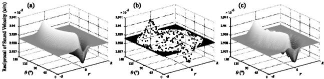
**Fig. 3** Exact, acquired, and interpolated projection data at r- $\theta$  surface. (a) Exact projection data. (b) .Original projection data. (c) Interpolated projection data.
