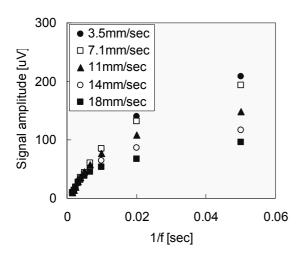
**Figure 2.** Inverse of chopping frequency (f) dependence of signal amplitude (flow rate=3.5-18mm/sec)
