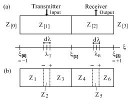
Fig. 1 (a) Transmitter and receiver located on a 2N-layered system (in the case of N=1). (b) Representation of transmitter and receiver.
