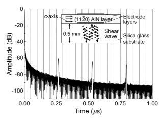
Fig. 4 Schematic diagram of pure thickness shear mode HBAR and impulse response of the resonator. Longitudinal and shear waves propagate in the 0.5-mm-thick silica glass substrate at respective velocities of 3770 m/s and 5960 m/s so that their echoes should be observed at 168 ns and 265 ns, respectively.
