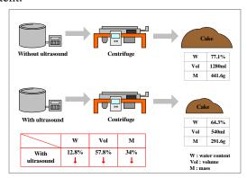
Fig. 4. Cake reduction due to ultrasound
