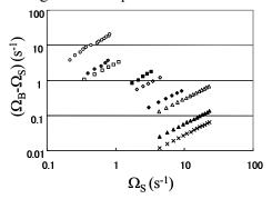
Fig.2 Relation between ( $\Omega_B$ - $\Omega_S$ ) and  $\Omega_S$  obtained for various viscosities. The viscosities are 5, 10, 50, 100, 500, 1000, 5000 and 10000 cP, respectively, from top to bottom.
