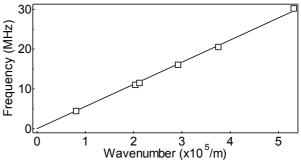
Fig. 5 Dispersion relation of acoustic phonon in air obtained with the millisecond Brillouin spectroscopy over the wavenumber range from  $k = 8.1 \times 10^4 \text{ m}^{-1}$  to  $k = 5.3 \times 10^5 \text{ m}^{-1}$  at 300 K. The experimental points ( $\Box$ ) are well fitted by a straight line, of which the gradient yields the phase velocity, 350 m/s for air
