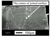
(c) The joined surface of the foil of pressed side.
