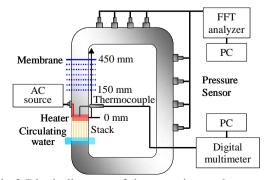
Fig.2 Block diagram of the experimental system.
