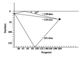
Fig. 3 Ray traces from source to receiver.
