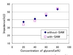
Fig. 8 Impedance spectrum of glycerol/water mixtures without-SAW and with-SAW.
