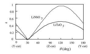
Fig. 2 Coupling constant of parallel field excitation.
