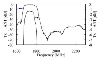
Fig. 4 Tx characteristic of the SAW duplexer
