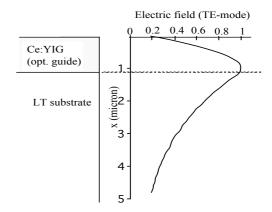
Fig. 4 Electric field distribution of TE-mode. (Calculated)
