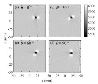
Fig.4 The images of internal crack reconstructed from the simulation. D = 10 mm. (a), (b), (c) and (d) show results of  $\theta = 0$ , 30, 60 and 90 °
