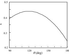
Fig. 4 Effective electromechanical coupling constant of SMR.
