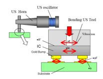
Fig. 1 Schematic diagram of IC chip bonding.
