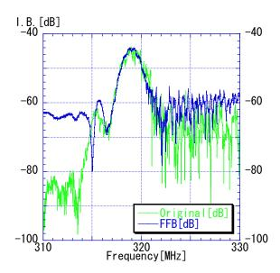
Fig. 5 Frequency characteristics of SAW devices after face to face bonding.
