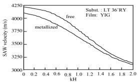
Fig. 2 Dependency of SAW velocity on Ce:YIG film thickness.
