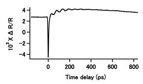
Fig. 3 Relative reflectivity change versus the time delay between the pump and the probe pulses. The nanopillar has a height of 290 nm and a width of 180 nm.
