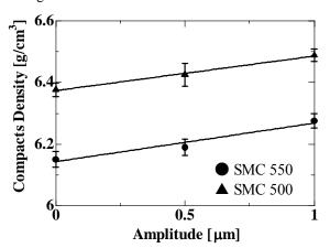
Fig. 7 Density vs. the vibration amplitude of the compaction die.
