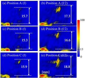
Fig. 3. Dependence of the SPACE images of the SCC on the measurement positions. (a) Fundamental and (b) subharmonic images at position A. (c) Fundamental and (d) subharmonic images at position B. (e) Fundamental and subharmonic images at position C.
