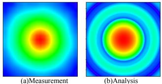
Fig. 5 Sound field distribution with cross section for axial distance in focal point
