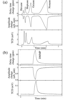
Fig.4 Responses of ball SAW sensor and TCD for detecting four mixed higher hydrocarbons (a) and DMMP (b).
