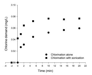
**Fig.2.** Chlorine demand of chlorination alone and chlorination with sonication
