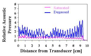
Fig. 3: Acoustic pressure distribution at 448 kHz, relative to the first antinode at the liquid surface for saturated water.
