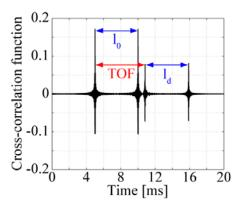
Figure 2: The cross-correlation function of the transmitted two LPM signals and the LPM signal
