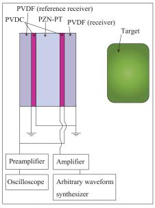
Fig. 1 : Proposed inline transmitter/receiver system.
