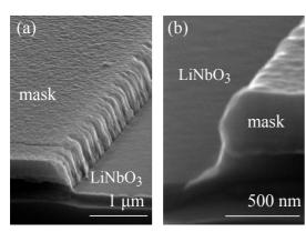
Fig.2 SEM images after the ion milling and RIE
