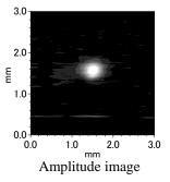
Fig. 6 PA amplitude image and signal distribution for the specimen with compound weld defect (modulation frequencies: 450Hz)
