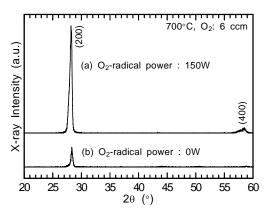
Fig. 2 XRD patterns of Ta<sub>2</sub>O<sub>5</sub> thin film deposited by O<sub>2</sub>-radical power of (a) 150 W and (b) 0 W.
