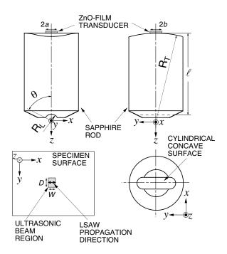
Fig. 1. Illustration of micro-LFB device and measurement region on specimen surface.
