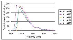
Fig 3 Input signal frequency vs. RPM
