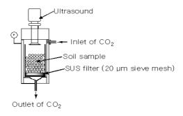
Fig. 3 Structure of the high pressure extractor.
