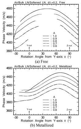
Fig. 2 Calculated phase velocity.
