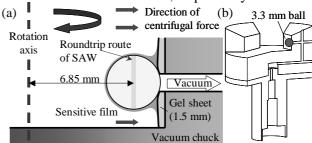
Fig.2 Schematic diagram of off-axis spin coating method (a) and cross-section drawing of the vacuum chuck (b)
