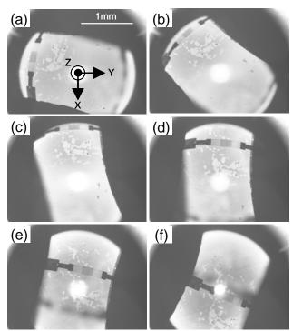
Fig. 5 Rotation of a ball SAW device. (a) At start. (b) After LB2 mode for 2.2s from (a). (c) After LB2 mode for 4.4s from (a). (d) After D3 mode for 3s from (c). (e) After D3 mode for 6s from (c). (f) After D3 mode for 9s from (c).
