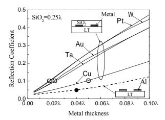
Fig. 3 Calculated reflection coefficients on flattened SiO<sub>2</sub>/various electrode/36°Y·X-LiTaO<sub>3</sub> and Al/36° Y·X-LiTaO<sub>3</sub> as function of electrode thickness.
