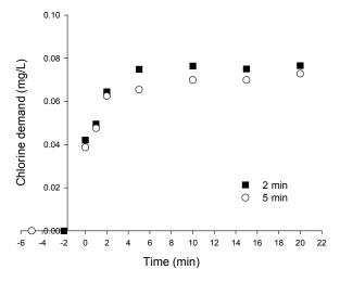
Fig. 3 Chlorine demand for 2 min and 5 min sonication
