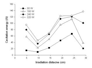
Fig. 2 Cavitation energy distributions for 80, 160, 240 and 320 W in the large-scale sonoreactor
