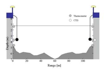
Fig. 1 Propagation area and arrangement of experimental equipments.
