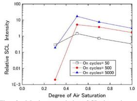
Fig. 2. Maximum relative SCL intensity vs. degree of air saturation for the cases of on-cycles = 50, 500 and 5000.
