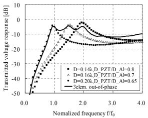
Fig. 6 Transmitted voltage response for the transducers array having differential connections calculated by FEM analysis.
