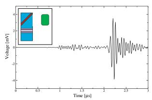
Fig. 3: Difference voltage between two PVDF films using Type-2 structure with a target stainless
