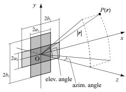
Fig. 1 Geometry of the coordinate system, rectangular array sound source and a reflection point P.
