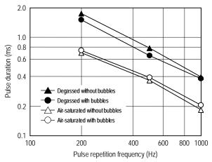
Fig. 4. Thresholds of PDs and PRFs for free radical production in air-saturated and degassed test solutions with and without microbubbles.
