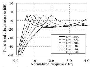
Fig. 5 Theoretical transmitted voltage response by FEM analysis when changing the diameter of the disk bender transducer.
