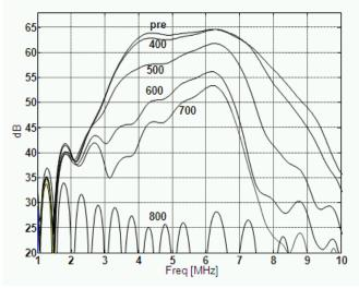
Fig.3 Round-trip responses after 120V driving. Numbers in the graph indicate cycle numbers of driving burst waves.
