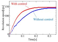
Fig.5 Comparison of transient response of revolution speed by presence of preload control.
