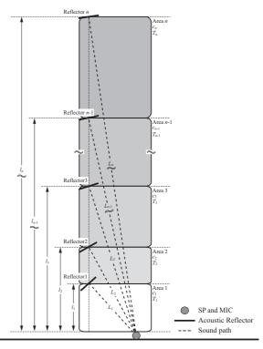
Fig. 1 Schematic of a measurement of temperature distribution using sound probes with reflectors.
