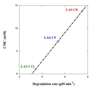
**Fig. 3** Relationship between degradation rates which have peaks in Fig. 2 and CMC of each LAS.
