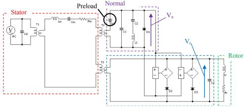
Fig.6 Equivalent circuit which can be simulated on a commercial circuit simulator.
