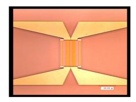
Fig. 3 Microscope photo of fabricated device.  $(400 \mu m \times 700 \mu m)$
