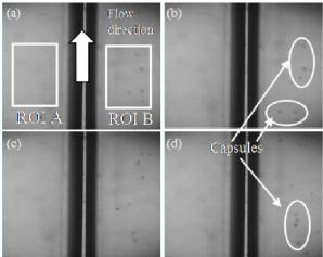
**Fig.3** Time series images of the observed area by 500 [fps] after injection of capsules suspension with ultrasound emission.
