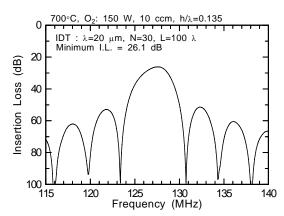
Fig. 3 Frequency response of IDT/Ta<sub>2</sub>O<sub>5</sub> thin film/fused quartz sample (c).
