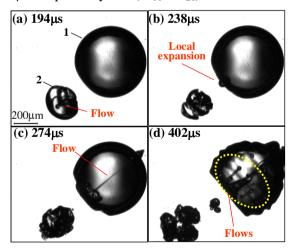
Fig.4 Several micro-flows generation.  $R_{1o}$  and  $R_{2o}$  are 338  $\mu m$  and 110 $\mu m$  respectively. L/(  $R_{1o}$  +  $R_{2o}$ ) is 1.26.
