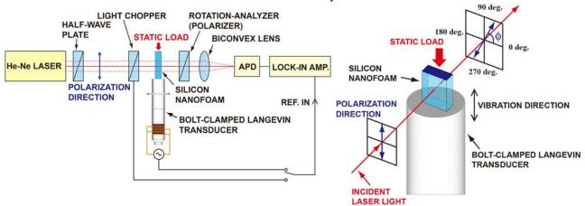
Fig. 1 Experimental set up for measuring the rotation angle of polarization in the laser light transmitted through a loaded silicon nanofom.
