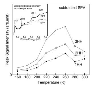
Fig. 1 Temperature dependence of subtracted SPV signal intensities at 1HH, 2HH and 3HH peaks. The insets show the subtracted PPT and SPV spectra at room temperature from Ref.1.
