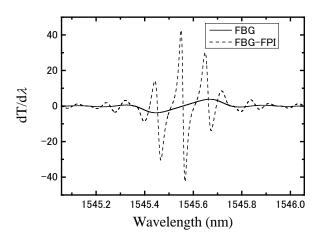
Fig. 4 Slope of transmittance spectra of FBG and FBG-FPI.
