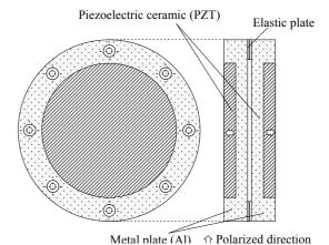
Fig. 1 Plane view and cross-sectional view of a disk bender transducer.
