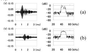
Fig.4 Receiving signals of target at (0, 50, 100) corresponding to (a): Chirp wave; (b): Adaptive signal.
