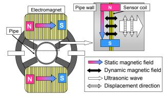
Fig.4 Drive principle of an EMAT for a T-mode pipe wave
