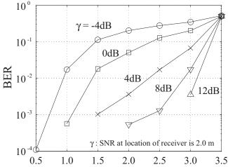
Location of receiver and noise source Fig. 3 BER performance with only transmitter-A.
