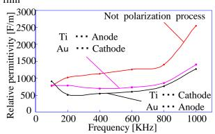
Fig.6 Effects of polling process on dielectric constant of bimorph type vibrator with hydrothermally synthesized PZT polycrystalline film
