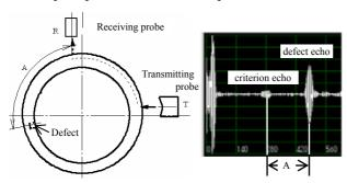
Fig. 3 The tandem method and the echo pattern
