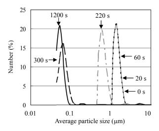
Fig. 3 Change in particle size distribution of nanometer-sized diamond particles by ultrasound exposure
