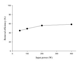
Fig. 3 Diesel removal efficiency for various input powers
