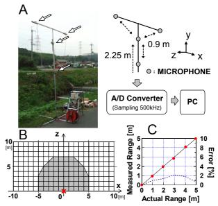
Fig. 1 (A) Four-microphone array system. Open arrow indicates the position of each microphone. (B) Theoretical range error of the microphone array system. The error was estimated to be less than 10 cm (gray area). Cross mark indicates the position of the microphone array. (C) Calibration measurement for the microphone array. Circles indicate the measured ranges and dotted line indicates the position error (see text).
