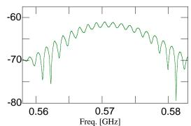
Fig. 3 Frequency characteristics of AlGaN/GaN SAW device used 2 DEG as electrodes.
