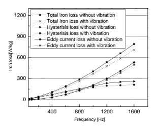
Fig. 4 The iron-loss according to frequency with and without vibration action
