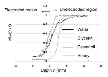
Fig. 4 Variations in normalized G vs. depth h for 4 different liquids.
