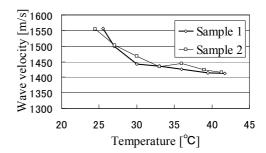
Fig. 7 Temperature dependence of observed wave velocity.
