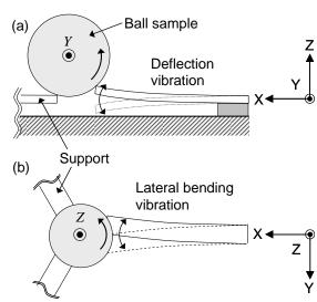
Fig. 1 Principle of rotation of a ball using cantilever. (a) Deflection mode. (b) Lateral bending mode.
