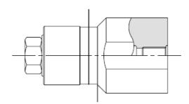
Fig.1 Schematic diagram of the bolt-clamp Langevin transducer (BLT).
