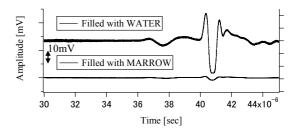
Fig. 8 Experimentally observed waveform passed through specimen.
