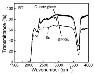
Fig. 3 FTIR spectra before and after UV-light irradiation
