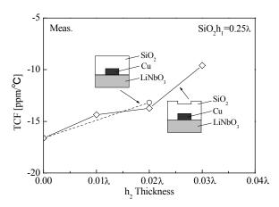
Fig2. Temperature coefficient of frequency as a function of  $\mathbf{h}_2$  thickness
