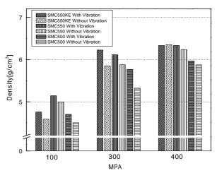
Fig. 3 The compact density obtained by ultrasonic acting and conventional compaction
