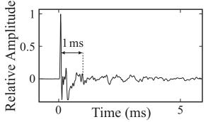
**Fig.1** Impulse response observed from performance evaluation system.
