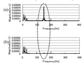
Fig.7 Vibration velocity vs. frequency at ground surface used noise wave (a) On buried object (b) Out of buried point
