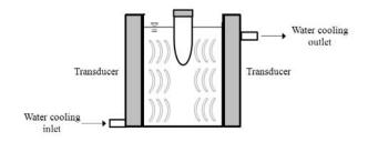
Fig. 1 Schematic of reactor
