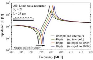
Fig. 1 Simulated impedance of a Lamb wave resonator on AlN using different interpolation schemes.
