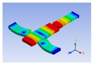
Fig. 4 Longitudinal vibration mode of the ultrasonic motor with holding mechanism.
