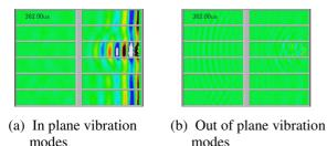
Fig.4 Emphasized reflected wave from circumferential defect in pipe.
