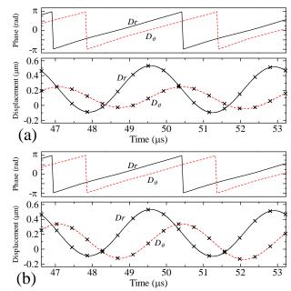
**Fig. 4** Time series representation of surface particle motion for low frequencies by decomposing locus in Fig. 2 into two components. (a) indicates outer surface and (b) indicates inner surface.
