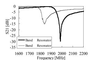
Fig. 1 Characteristics of SAW resonator
