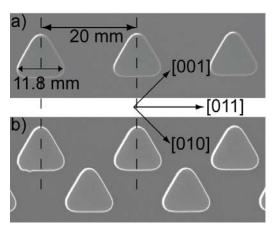
Fig. 1 SEM images of rectifier samples. a) Single row structure and b) Double row structure.
