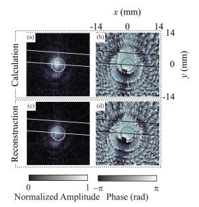
Fig. 2 Experimental results of reconstructed and calculated sound fields. (a) and (b) the calculated sound fields; (c) and (d) the reconstructed sound fields. (a) and (c) the amplitude of sound fields; (b) and (d) the phase.
