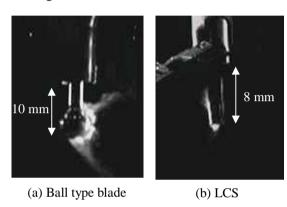
Fig.3 Cavitation.bubble from blades.
