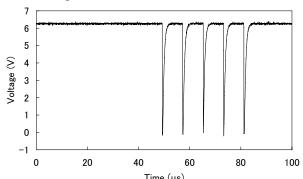
(b) Output of the Receiver Side comparator.
