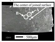
(b) The joined surface of the foil of SAW device side.
