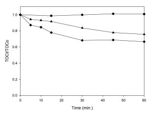
**Fig. 3.** TOC degradation for tannins with individual and combined schemes (0.100 L, 25  $\pm$  3°c, [C<sub>76</sub>H<sub>52</sub>O<sub>46</sub>] = 0.3 mM); •, US only (170 kHz, 400 W); •, O<sub>3</sub> only (1 g L<sup>-1</sup>); •, US + O<sub>3</sub>)
