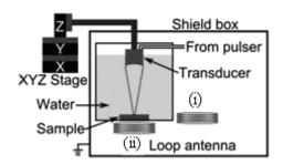
Fig.1 Schematic diagram of measurement setup.
