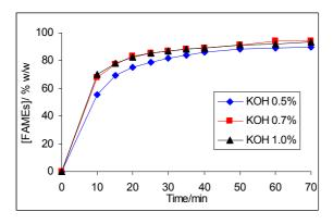
Fig.3 Effect of KOH catalyst amount on the conversion of FAMEs. Molar ratio of oil to methanol was 1:5
