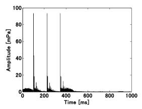
Fig. 2 Correlated signal using code '3265'.
