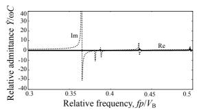
Fig. 3 Input admittance of infinitely-long Cu IDT
