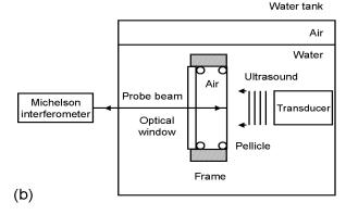
Fig. 1 Two methods for underwater ultrasound detection using a Michelson interferometer: (a) Transmission method and (b) Reflection method.
