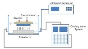
Fig. 1 Schematic of sonochemical reactor
