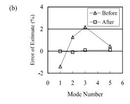
Fig. 3 Errors of the estimated capacitance ratio before and after the correction of  $g_n$ , in the cases of (a) L-effect and (b) T-effect for #1.
