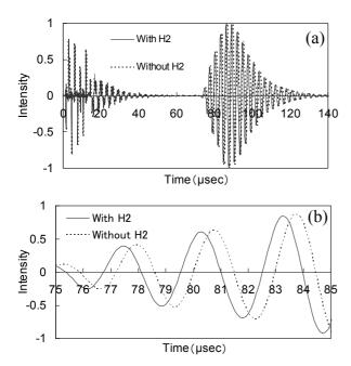
Fig.2 (a) Signal intensity form the ultrasonic receiver. Four pulses of sound wave traveled after 28mm of distance are shown. (b) Enlargement of Fig. 2(a).
