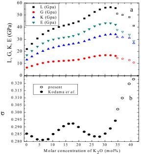
Fig. 4 The composition dependences of (a) L, G, K, E and (b)  $\sigma$ .
