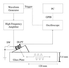
Fig. 2. Experimental setup.
