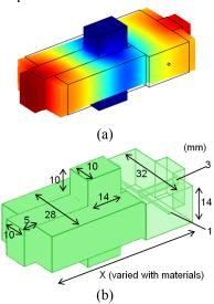
Fig. 3 Desired mode & dimensions of final welding horn.
