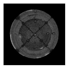
Fig.7 Example of C-Mode image of phantom.
