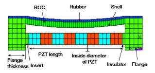
Fig. 1 Finite element model of the transducer
