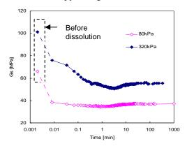
Fig. 4. Evolution of small strain shear modulus during dissolution.
