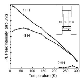
Fig. 2 Temperature dependence of 1HH, 1LH, and 2HH PL peak intensities
