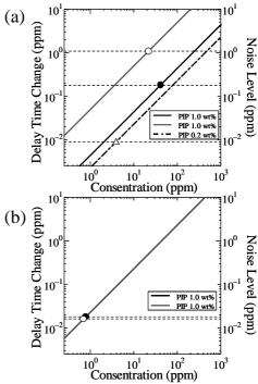
Fig.5 Detection efficiencies and noise levels of delay time change for DMMP obtained with sensors coated by conventional spin coating method (a), and off-axis spin coating method (b). Positions of slope show efficiencies and dashed lines show noise levels. Circles and triangle show detection limits.
