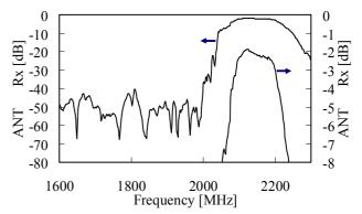
Fig. 5 Rx characteristic of the SAW duplexer
