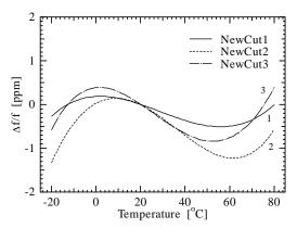
Fig. 2 Theoretical analyses results of frequency-temperature characteristics
