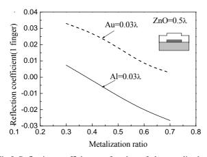
Fig.5 Reflection coefficient as function of the metalization ratio.
