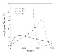
Fig. 3 Coupling coefficient for free surface calculated by the Green's function method.
