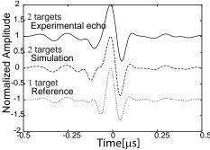
Fig. 3 The echo from a polyethylene sheet 0.05 mm thick, the pseudo echo  $s_1(t)$ , and the echo from an acrylic board.
