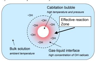
Fig. 1. Effective reaction zone where the sonochemical reaction take place.
