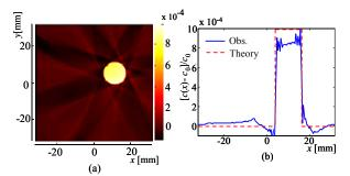
**Fig.4** Reconstructed sound speed image of the cylindrical object: (a)gray scale image on (x,y) plane, (b)cross-sectional image on x-axis. Results from the scattered data (solid line) are compared to the theory (dotted line).
