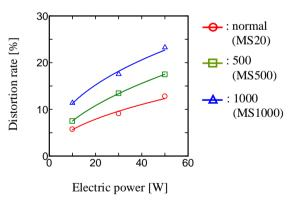
Fig. 5 Relationship between Electric power and Distortion rate.
