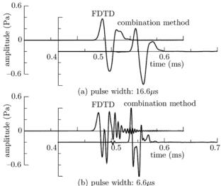
Fig.3 Calculated waveforms reflected from the target.
