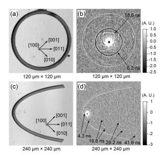
Fig. 2. (a) Optical reflectivity image of a circular resonator of internal diameter  $100~\mu m$ . (c) Optical reflectivity image of a sample with a parabolic boundary. The substrate is a Si (001) covered with a 40 nm polycrystalline Cr film. (b), (d) snapshots of the SAW propagation corresponding to the samples of (a) and (c), respectively. The times after pumping are indicated by the arrows.
