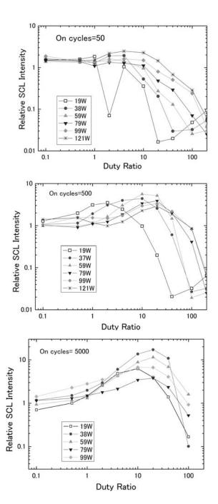
Fig.1. Relative SCL intensity as a function of duty ratio (= off cycle number/on cycle number) for (a) on-cycles=50, (b) on-cycles=500, and (c) on-cycles= 5000.
