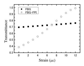
Fig. 6 Strain dependence of transmittance of FBG and FBG-FPI.
