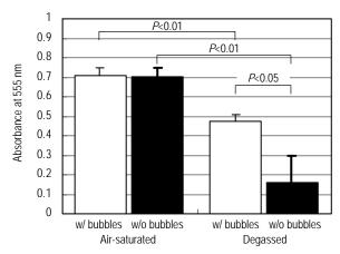
Fig. 2. Comparison of the amounts of free radicals produced in air-saturated and degassed solutions with and without microbubbles. Bars and error bars show the mean  $\pm$  S.D. (n=4).
