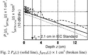
Fig. 2  $P_{\alpha}(z)$  (solid line),  $I_{\text{SPTA}}(z) \times 1 \text{ cm}^2$  (broken line) and  $I_{\text{SATA1}\times 1}(z) \times 1 \text{ cm}^2$  (dashed line) for 3.5-MHz ultrasonic field radiated from 14-mm-diameter plane circular transducer.
