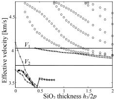
Fig. 6 Variation of the effective velocities of acoustic waves with  $h_2/2p$  (Controlled: Al  $h_1$ = $h_3$ =0.16 p)
