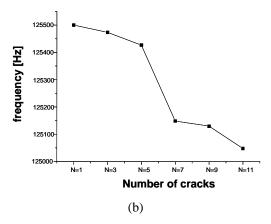
Fig. 3 Oscillation frequency change in relation to the (a) crack length and (b) crack number
