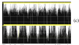
Fig.2. Oscilloscope tracings of SL pulses. Upper: Na emission. Lower: Continuum emission. Applied voltage are (a)16.5 Vpp, (b) 23.5 Vpp, and (c) 35 Vpp.
