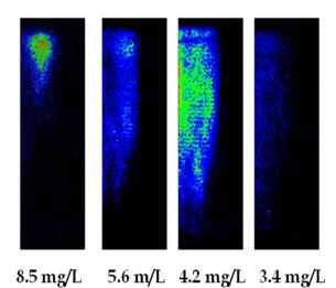
Fig. 2 Sololumonescence structure at different dissolved oxygen concentration. Continuous sonication at 448 kHz and 22 W.
