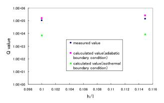
Fig.2 Comparison between calculated and measured Q value as a function of the parameter h/l
