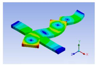
Fig. 5 Bending vibration mode of the ultrasonic motor with holding mechanism.
