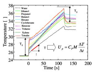
Fig. 2 The energy conversion for different solvents.
