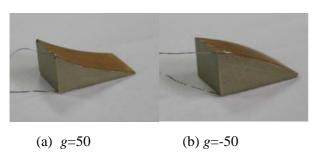
Fig. 2. Photograph of piezoelectric vibrators with exponentially tapered thickness.
