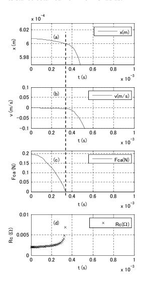
Fig.3 Behavior of the contact at early stage of break in real values. (a) Displacement x. (b) Velocity v. (c) Contact force  $F_{ca}$ . (d) Contact resistance  $R_c$ .
