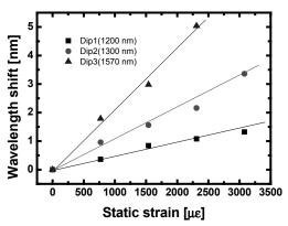
Fig.3. Strain-induced wavelength-shifts for Dip1, Dip2 and Dip3.
