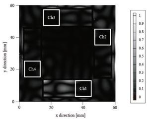
Fig. 3 Vibration distribution of the stage at 69 kHz.
