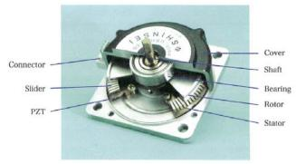
Fig 1 Ultrasonic motor USR60E3
