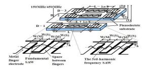
Fig. 1 Proposed SAW gas sensor for "Sensor Network" system
