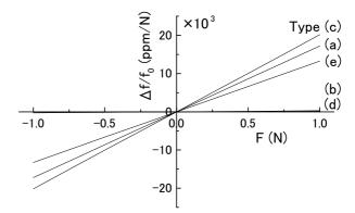
Fig. 4 Calculated characteristics of  $F-\Delta f/f_0$  of force sensor.
