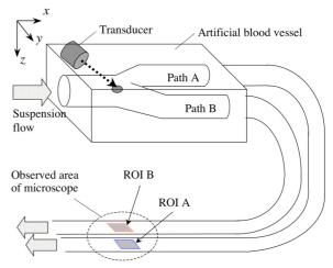
**Fig.1** Experimental setup including artificial blood vessel.
