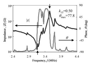
Fig. 1 Frequency dependence of impedance, Z, in the (15) mode for KN-Mn0.1.
