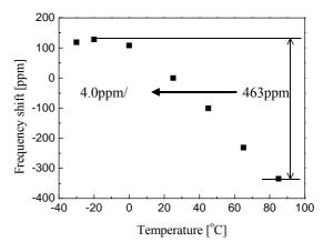
Fig.8 Frequency shift of the fabricated filter relative to temperature.
