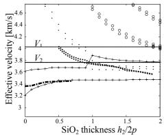
Fig. 5 Variation of the effective velocities of acoustic waves with  $h_2/2p$  (Flattened: Cu  $h_1$ =0.2 p)
