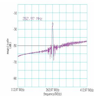
Fig. 1. The measured frequency response of the SAW filter for ST-cut quartz substrate with electrode width of 3  $\mu m$ .
