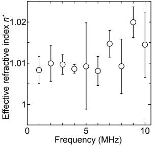
Fig. 2 Measured effective refractive index for far-field ultrasound (Light wavelength = 633 nm, Water temperature = 22.0°C).
