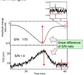
Fig.3 Excellent sensitivity of ball SAW sensor to tridecane
