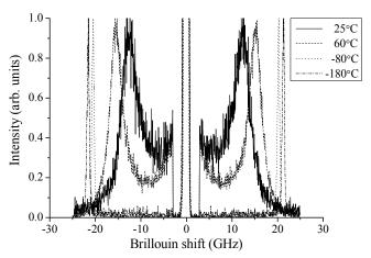
**Fig. 3** Observed Brillouin spectra of a HEWL crystal at 25°C(line), 60°C(broken line), -80°C(dotted line), -180°C (chain line), which include the scattering from the longitudinal acoustic phonon.
