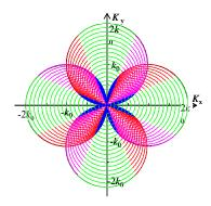
**Fig.2** Contour plots of the data in the Fourier plane with multi-frequency wave illumination from quadrangular direction.
