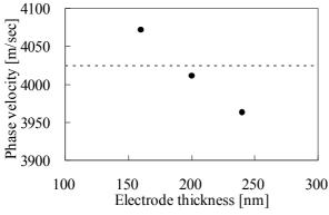
Fig. 3 A phase velocity dependence of the electrode thickness
