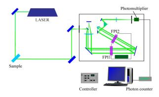
Fig. 1 Schematic diagram of the micro-Brillouin scattering apparatus.
