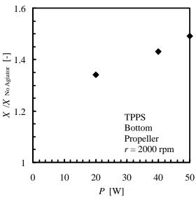
Fig.3 Effect of electrical power to transducer on ratio of TPPS decomposition conversion with agitator
