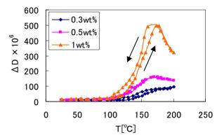
Fig. 5 Temperature dependence of  $\Delta D$  of PS films.
