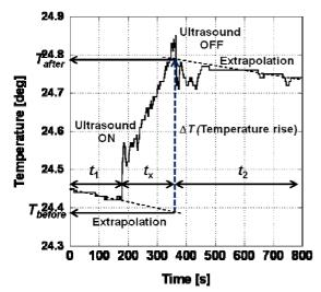
Fig. 3 Method of measuring the temperature rise caused by ultrasonic irradiation.
