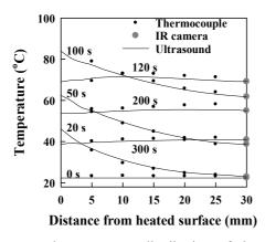
Fig. 1 Internal temperature distribution of the steel plate and its variation during heating and cooling.
