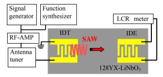
Fig. 6 Mixing and Sensing device.
