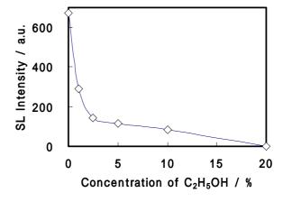
Fig. 6 Addition effect of ethanol on MBSL
