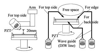
(a)Spot type (b)Waveguide type Fig.2 Application of waveguide type transducer to the spin cleaning unit
