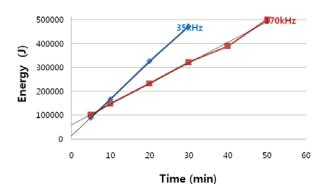
Fig. 3. Cavitation energy according to frequency
