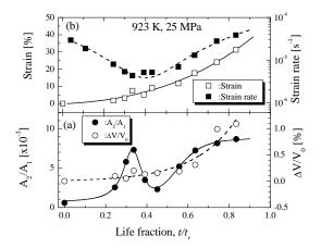
Fig. 3 Relationship between  $A_2/A_1$ ,  $\Delta V/V_0$ , the creep strain, the strain rate, and life fraction,  $t/t_r$ .
