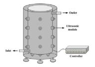
Fig. 1. Large scale ultrasonic processor
