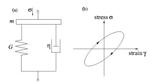
Fig. 1 (a) Mechanical model. (b) Stress-strain relationship.
