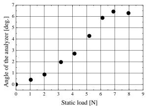
Fig. 3 Angle of the analyzer vs. static load.
