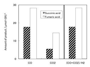
**Fig.4** Comparison of sonolytical rates between saturated and unsaturated dicardoxylic acids
