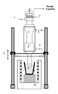
1. Cooling air in, 2.PZT 3. Booster horn, 4. Radiator horn, 5. Cooling water out, 6. Cooling water in, 7. Elevator, 8. Melts, 9. Graphite crucible, 10. Electric resistance furnace
