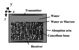
Fig.6 FDTD simulation model.
