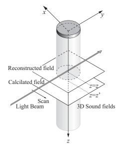
Fig. 1 Schematic of sound velocity measurement using Optical-CT and coordinate system.
