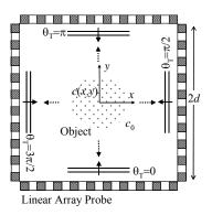
**Fig.1** Data observation geometry using four linear arrays along square perimeter of the object.
