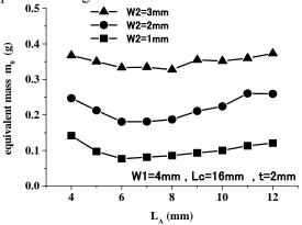
Fig.5 Calculated relationship between L<sub>A</sub> and m<sub>0</sub>.
