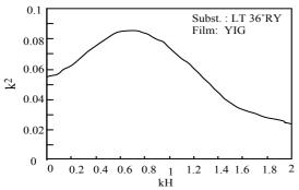
Fig. 3 Dependency of coupling constant on Ce:YIG film thickness
