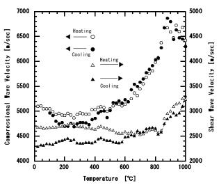
Fig.2. Temperature dependence of compressional wave velocity ( $\bigcirc$ :Heating,  $\bullet$ :Cooling) and shear wave velocity ( $\triangle$ :Heating,  $\blacktriangle$ :Cooling).
