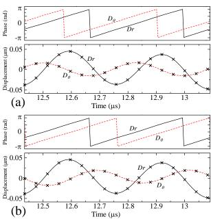
**Fig. 5** Time series representation of surface particle motion for high frequencies by decomposing locus in Fig. 3 into two components. (a) indicates outer surface and (b) indicates inner surface.
