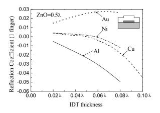
Fig.2 Reflection coefficient (1 finger) of ZnO/various IDT/27°YX quartz as function of IDT thickness at ZnO thickness of  $0.5\,$
