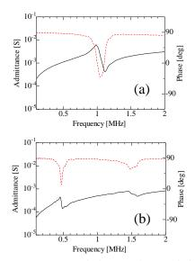
Fig. 1. Frequency-Admittance characteristics of DLPT electrically connected (a) in Parallel and (b) in series. Solid lines indicate the absolute value of admittance and dotted line the phase of admittance.
