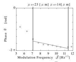
Fig.3 Relation between  $\theta$  and  $\sqrt{f}$  in the 28 $\mu$ m.
