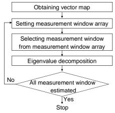
Fig. 2 Flowchart for computing scalar component
