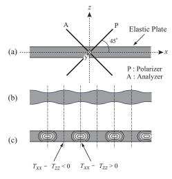
Fig. 2 Photoelastic optical system and visualized image of elastic wave.
