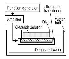
Fig. 1. Experimental setup used in the experiments.
