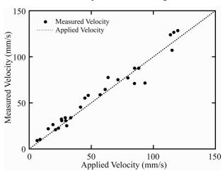
Fig.4 Relationship between applied velocity and measured velocity.
