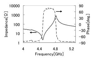
Fig. 5 Measured impedance and phase characteristics near  $A_1$  mode of Lamb wave response( narrow range)
