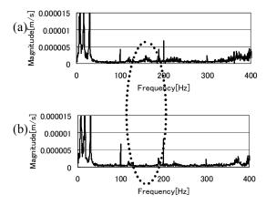
Fig.6 Vibration velocity vs. frequency at ground surface used noise wave (a) On buried object (b) Out of buried point
