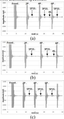
**Fig. 2** Typical pulse-echo signals from the steel specimen (a) at 20 mm thick and (b) at 25 mm thick, and (c) aluminum specimen at 20 mm thick.
