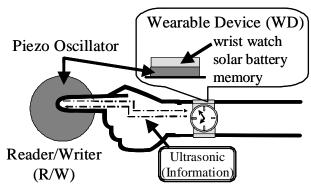
Fig. 1 Communication System for Wearable Device.
