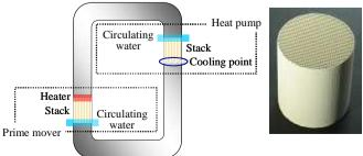
Fig.1 Schematic view of the loop-tube and a photograph of a stack.
