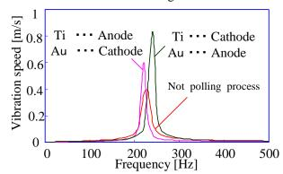
Fig.5 Effects of polling process on vibration velocity of bimorph type vibrator with hydrothermally synthesized PZT polycrystalline film
