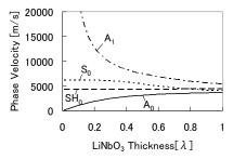
Calculated phase velocities of plate waves as a function of LiNbO3 thickness
