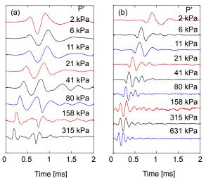
Fig. 1 Measured shear wave signatures: (a) Incheon ; (b) Busan.
