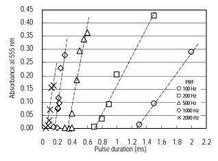
Fig. 3. Relationship between PDs and amounts of free radicals produced in air-saturated test solution without microbubbles.
