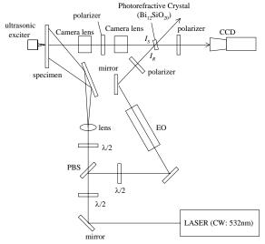
Fig. 1 Experimental setup
