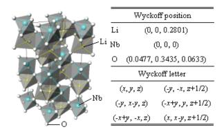
Fig. 1 Crystalline structure and Wyckoff position of LiNbO<sub>3</sub>.
