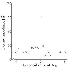
Fig.3 Relationship between numerical value of  $N_{\rm W}$  and electric impedance.
