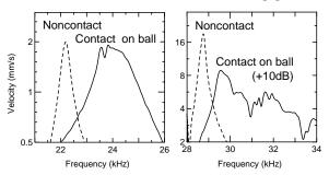
Fig. 3 Vibration spectra of free end of a cantilever. (a) Deflection vibration. (b)Lateral bending vibration.
