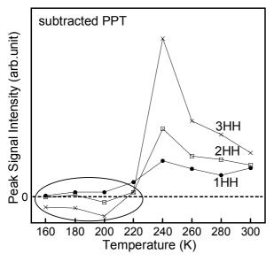
Fig. 2 Temperature dependence of subtracted PPT signal intensities at 1HH, 2HH and 3HH peaks.
