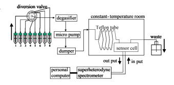
Fig. 1 Homebuilt flow injection system
