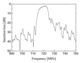
Fig.7 Frequency Characteristic of the fabricated filter.
