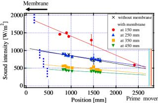
Fig.3 Distribution of sound intensity; at 400 sec. after heat supply started.
