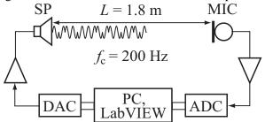
**Fig.3** Block diagram of a performance evaluation system of acoustic communication in the air.
