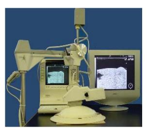
Fig. 1 Ultrasound diagnostic equipment.
