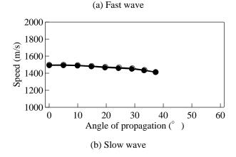
Fig. 3 Fast and slow wave speeds in stratified trabecular phantoms without and with trabecular rods vs. propagation angle to trabecular plates.
