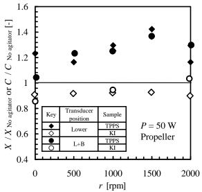
Fig.5 Effect of revolution rate on ratio of TPPS decomposition conversion or  $I_3^-$  concentration for dual irradiation with agitator
