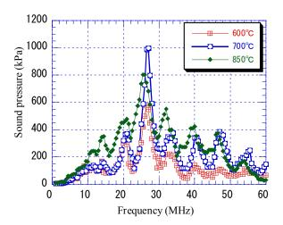
Fig. 1 The frequency characteristics of the sound pressure using each ultrasound probes
