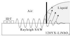
Fig 1. Schematics of SAW steaming
