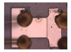
Fig. 2 Optical micrograph of the FBAR
