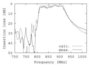
Fig. 4 Frequency response of fabricated DMS filter.
