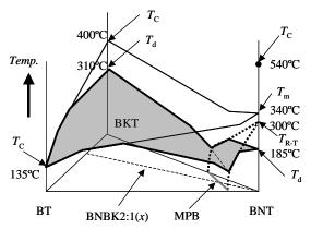
Fig. 2 The phase relations of the BNT-BKT-BT system.
