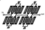
Fig. 2: Composition of RF filter composed of DMS.
