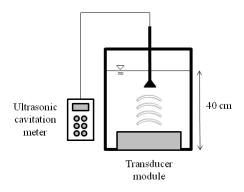
Fig. 1 Schematic of the large- scale sonoreactor
