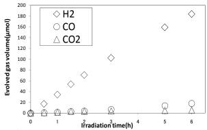
**Fig.1** Sonolytical products in gas phase from succinic acid solution at 25°C
