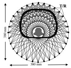
Fig.1 Transmitter/receiver arrangement and propagation path.
