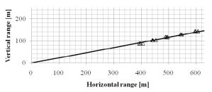
Fig.2 Relative position of the receiver. (0,0) as the transmitter position.  $\triangle$ : relative position of the receiver. Solid line: 77° from vertical.
