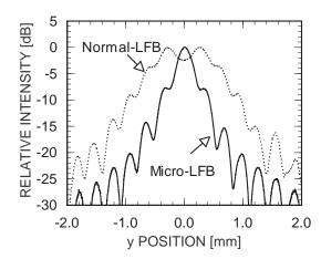
Fig. 2. Acoustic field along y-axis direction (ultrasonic frequency: 225 MHz, transducer width along y-axis direction: 1.50 mm).
