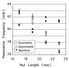
Fig.2 Resonance frequencies shift by changing nut length.
