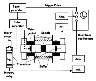
Fig.1. Schematic diagram of the apparatus for measuring ultrasonic velocity and attenuation even at high temperature region.
