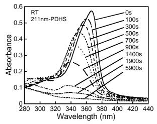
Fig. 1 Effects of UV-light irradiation on the OA spectrum of 211-nm-thickness sample
