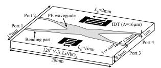
Fig. 1 Configuration of waveguide-type AOM.
