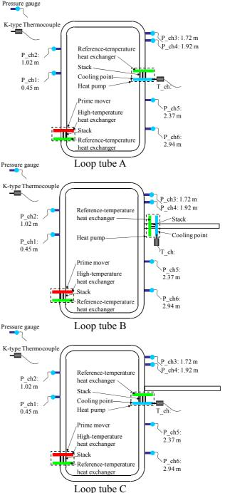
Fig.1 Schematic illustrations and the experiment setups of loop tubes A, B, and C.
