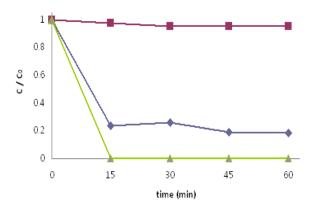
**Fig. 2** Degradation of C.I. Reactive Black 5 (■ : Sonochemical process,  $\spadesuit$  : Fenton process,  $\spadesuit$  : Sonochemical + Fenton process), reaction condition -  $H_2O_2 = 120 \text{mgL}^{-1}$ ;  $H_2O_2$ :FeSO<sub>4</sub> = 1:4; [dye]<sub>0</sub> =  $100 \text{mgL}^{-1}$ ; frequency = 35kHz; power = 400 W
