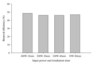
**Fig. 2** Diesel removal efficiency for various combinations of input power and irradiation times
