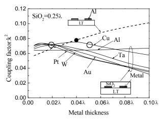
Fig. 4 Calculated coupling factors on flattened SiO<sub>2</sub>/various electrode/36°Y·X-LiTaO<sub>3</sub> and Al/36° Y·X-LiTaO<sub>3</sub> as function of electrode thickness.
