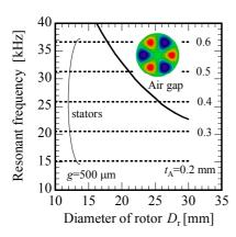
Fig. 3 Resonant frequency of stators and gap space as a function of rotor diameter calculated by FEM.
