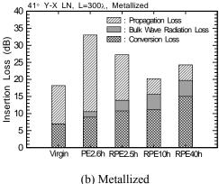
Fig. 4 Details of insertion loss of 41° Y-X LN sample.
