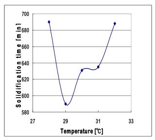
Fig.1. Solidification time dependent on temperature in the case of no ultrasonic irradiation
