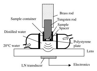
Fig.1. Experimental setup of acoustic system.
