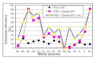
Fig. 4 Comparison of extraction efficiency of metal species from the soil samples using pure  $CO_2$ ,  $CO_2$  + Cyanex 272, and  $CO_2$  + Cyanex 272 + Ultrasound.
