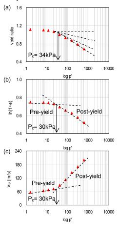
Fig. 2 Determinating preconsolidation stress at Incheon site: (a) Casagrande; (b) Onitsuka; (C) shear wave method.
