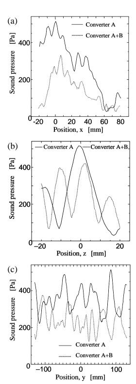
Fig. 3 Distribution of sound pressure in the vicinity of the converging point. (a): in the direction of the x-axis, (b): in the direction of the y-axis.
