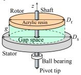
Fig. 1 Construction of non-contact type ultrasonic motor using a flexurally vibrating disk.
