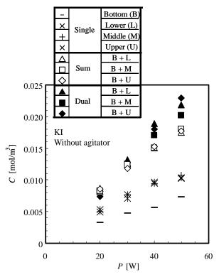
Fig.2 Effect of electrical power to one transducer on the I<sub>3</sub> concentration for different positions of transducers
