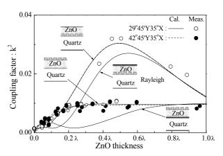
Fig.1 Electromechanical coupling factor of ZnO/quartz as a function of ZnO thickness.
