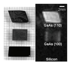
Fig.2 Photograph (left) and ASEM image (right) of GaAs (110), GaAs(100) and Si(100) plates.
