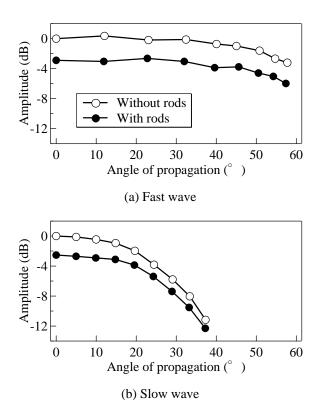
Fig. 2 Fast and slow wave amplitudes in stratified trabecular phantoms without and with trabecular rods vs. propagation angle to trabecular plates.
