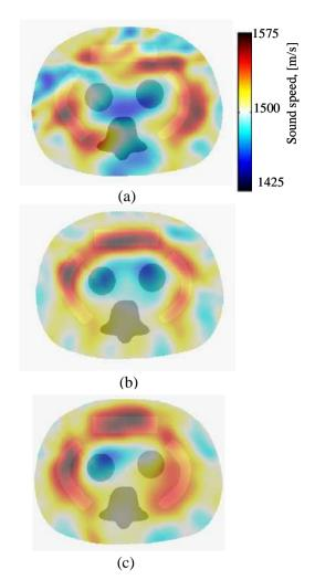
Fig.3 Reconstructed sound speed image of the abdominal phantom: (a) image using the measured data, (b) image using the simulated data based on the straight ray propagation model, (c) same as in (b) based on the finite difference calculation. The reconstructed colored sound speed images are superimposed with the predetermined gray-scale image.
