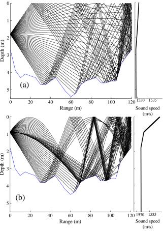
Fig. 3 Rays calculated by Bellhop under the parameters of temperature and depth at (a) 6:00 and (b) 14:00 on August 16, 2007. Graph on the right side shows sound speed profile in the water used for calculation.
