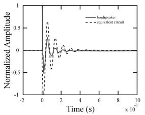
**Fig.4** Impulse response of loudspeaker and equivalent circuit.
