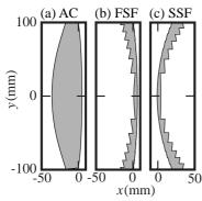
Fig. 3 Shapes of lenses. (a) Aplanatic Convex lens (AC), (b) First surface Stepped aplanatic Fresnel lens (FSF),
