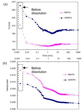
Fig. 3. Process monitoring during dissolution of vanishing materials at the vertical effective stresses of 80 kPa and 320 kPa: (a) Vertical strain versus time; (b) Shear wave velocity versus time.
