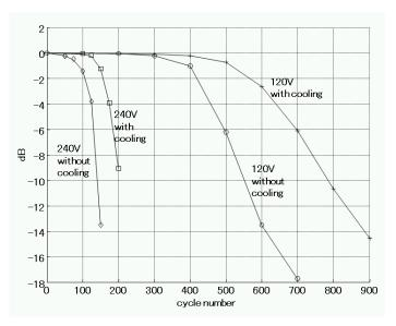
Fig.4 Sensitivity change of round-trip responses caused by breakdown
