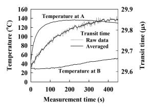
Fig. 3 Variations of the temperatures and the transit time of the SAW on the steel surface during heating.
