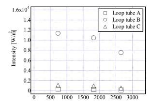
Distance from the heater [mm] Fig.3 Sound pressure distribution in the case of input heat energy of 330 W for loop tubes A, B, and C.
