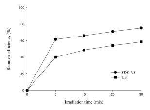
**Fig. 4** Diesel removal efficiency for only ultrasound and combination of ultrasound and surfactant
