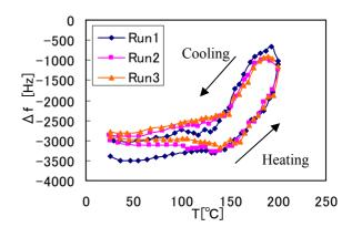
Fig. 3 Temperature dependence of  $\Delta f$  for PS film prepared with 0.5 wt% solution.
