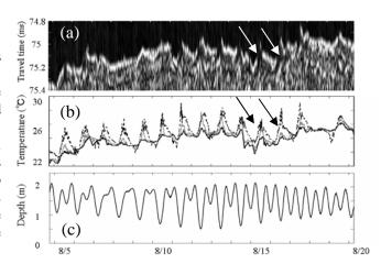
Fig.2 (a) Extracted amplitude of received signals correlated with M-sequence. (b) Water temperature at sea side. (Solid line) water temperature around seabed, (gray line) water temperature near the transducer, (dashed line) water temperature near the sea surface. (c) Distance between the surface and the transducer.
