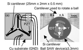
Fig. 2 Manipulator with three cantilevers. (a) Schematic illustration. (b) Ball SAW device on the manipulator.
