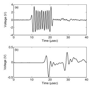
Fig. 2 Evolution of the transmitted toneburst for the intact sample (a) and the thermally damaged one (b).
