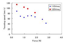
Fig.5 Traveling speed vs force characteristic (at 77kHz)
