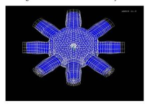
Fig. 3 Radial vibration mode by ANSYS.
