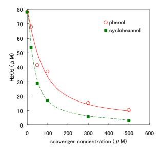
Fig.2. Changes in concentration of the sonochemically formed hydrogen peroxide in phenol and cyclohexanol aqueous solutions.
