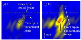
Fig. 5. Superimposition of the optical crack image on the SPACE images. (a) Fundamental and (b) subharmonic images.
