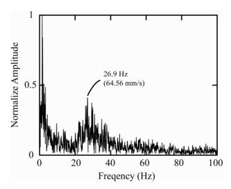
Fig.3 Example of a spectrum in the range of 0 Hz to 100 Hz from a photo-detected signal.
