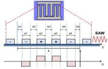
a1,a2,a3,a4: width of electrodes, b1,b2,b3,b4,b5: interval between electrodes, L: width of one section
