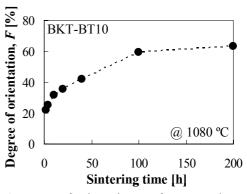
**Fig. 1** Degree of orientation, F, for textured BKT-BT10 sintered at 1080°C as a function of sintering time.
