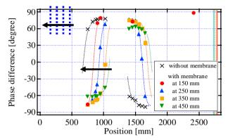
Fig.4 Distribution of phase difference between sound pressure and particle velocity; at 400 sec. after heat supply started.
