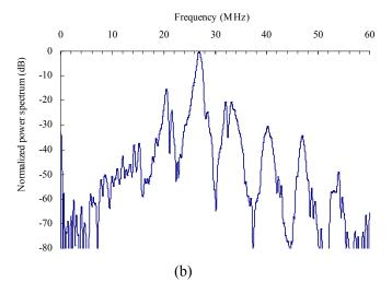
Fig. 2 (a) Received waveform and (b) normalized power spectrum of the irradiated ultrasound by the ultrasonic probes using PZT film annealed at 700 °C.
