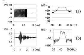
Fig. 2 (a): Chirp wave; (b): Reference receiving signal.
