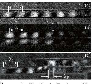
$\lambda_L$ : Wave length of Lamb wave (S<sub>0</sub>)  $\lambda_B$ : Wave length of Boundary wave
