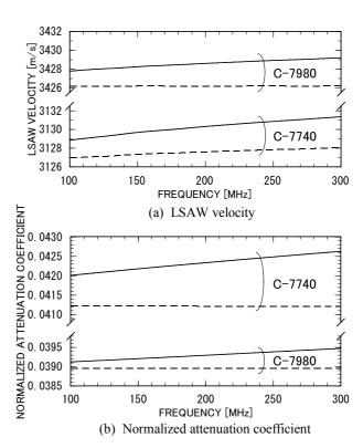
Fig. 2 Calculated results of LSAW propagation characteristics for C-7980 and C-7740. Solid lines denote the results considering the shear-wave component of water, broken lines denote the results treating water as an ideal fluid.
