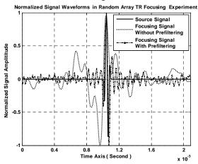
Fig.4. normalized signal waveforms of random array TR focusing experiment
