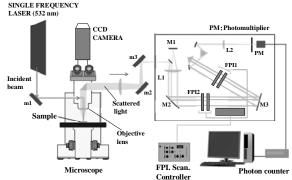
**Fig. 1** Schematic diagram of the micro-Brillouin scattering instrument<sup>2</sup>.
