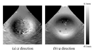
Fig. 5 Estimated displacement by 2D-CA method with hyperbolic scan
