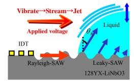
Fig. 5 Principal of SAW streaming.
