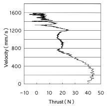
Fig. 3 Thrust-speed of V-shape motor
