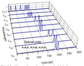
Fig.5 Incident pulse train of an optical label.
