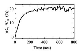
Fig. 3 Elastic constant change,  $\Delta C_{11}/C_{11}$ , calculated from measured frequency change,  $\Delta f/f_0$  of Ag thin film.
