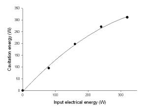
Fig. 3 Relationship between input electrical energy and measured cavitation energy for 35 kHz
