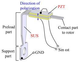
Fig.1 Basic construction of the stator of L-shaped ultrasonic actuator.
