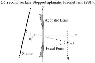
Fig. 4 Arrangement of the 2D FDTD analysis.
