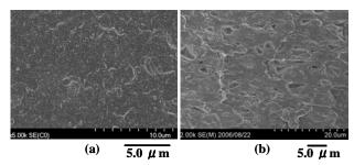
Fig. 3. SEM images of (a) ZnO-doped rubber ( $\times$  5000) and (b) conventional rubber ( $\times$  2000).
