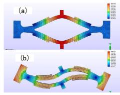
Fig. 4 The bending modes of the vibrator with rectangular counterweight and diamond hollow structure
