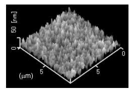
Fig. 4 AFM image for Ta<sub>2</sub>O<sub>5</sub> thin film sample (c).
