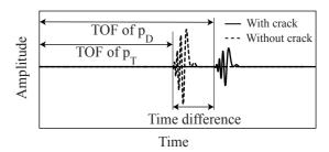
Fig.2 Times of flights (TOF) of p<sub>T</sub> and p<sub>D</sub>
