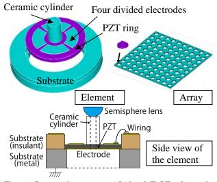
Fig. 1 Proposed structure of the MDOF ultrasonic actuator and the composition of the array.
