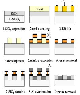
Fig.1 Fabrication process
