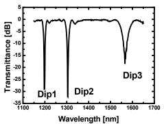
Fig.2. Typical transmission spectrum of LPG.
