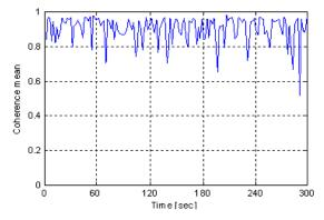
Figure 6. Mean coherence of all receivers with respect to temporal delay.
