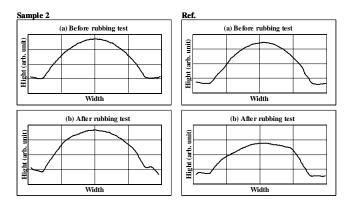
Fig. 2. Lens profiles of (left) ZnO-doped rubber and (right) conventional rubber (a) before and (b) after rubbing scanning test.
