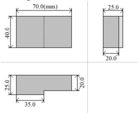
Fig. 1 Dimensions of the specimen used in the present work.
