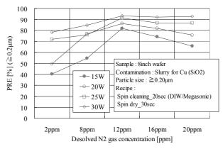
Fig. 4 Dissolved N<sub>2</sub> gas concentration dependence on particle removal efficiency changing the output power
