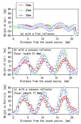
Fig. 3. Measured force on steel ball along the sound beam axis.
