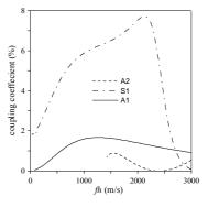
Fig.4 Coupling coefficient for metalized surface calculated by the Green's function method.
