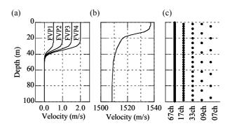
Fig. 2 (a) FVPs (b) SVP (c) TRA configurations.
