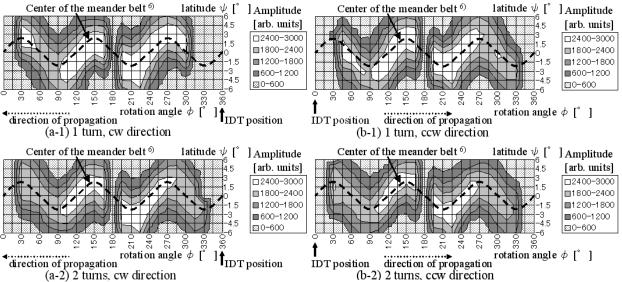
Fig. 3 Amplitude distribution of cw and ccw SAW propagation
