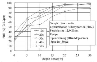
Fig. 3 Output power dependence on particle removal efficiency changing the cleaning time
