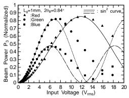
Fig. 5 Measured diffraction properties.
