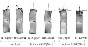
Fig.3 Load influence of the vibration resonance mode.(*W/L*=0.255)
