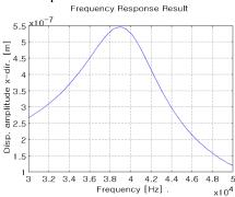
Fig. 4 Frequency response result of JPN horn.
