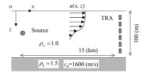
Fig. 1 Simulation condition.
