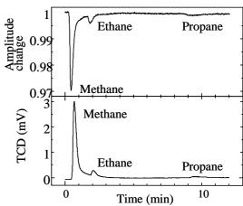
Fig.4 Response for Methane, Ethane, Propane a) Ball SAW Amplitude response b) TCD response
