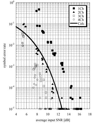
Fig.4 Symbol error rate vs average input SNR. (transmission rate: 80 kbps)
