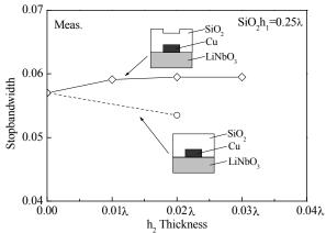
Fig4. Stopbandwidth as a function of h<sub>2</sub> thickness
