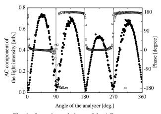
Fig. 4 Intensity and phase of the AC component of the laser light vs. the angle of the analyzer when 26-kHz sound wave is applied.
