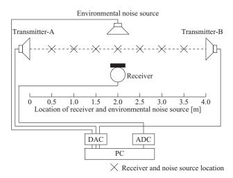
Fig. 2 System fabrication of the experiment system using DPSK digital acoustic communication and location of the two transmitters, the receiver and the environmental noise source.
