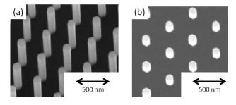
Fig.1 (a), (b) Typical scanning electron microscope images of GaAs nanopillars taken from different angles.
