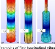
Fig. 1 Examples of first longitudinal vibration mode Ratios of front and back velocity amplitude are, (a):434/434=1.00; (b):538/374=1.44; (c):987/312=3.16
