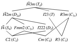
Figure 2. Group–subgroup relationship about the  $I\bar{4}3m$  ( $T_d$ ) symmetry. There are two subgroups that have tetragonal symmetry;  $D_{2d}$  and  $S_4$ .
