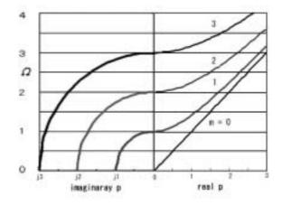
Fig. 1 Dispersion curves of SH waves in a plate
