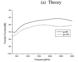
(b) Experiment Fig. 3. Power transfer function change with vibrator shape.
