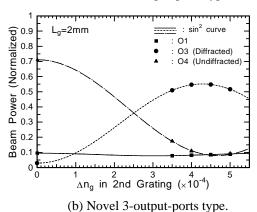
Fig. 2 Simulated diffraction properties.
