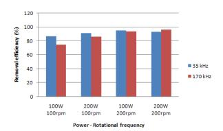
**Fig. 2.** Removal efficiency according to frequency, power, and rotational frequency
