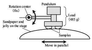
Fig. 1. Motion of abrasion tester.
