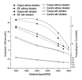
Fig. 6 The results of dynamic motor performance having SMC core both ultrasonic treated and no treated one
