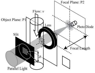
Fig.1 Configuration of a Fourier transform spectrometer
