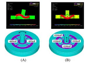
Fig. 2 Vibration modes of the stator and how to apply the voltages to the electrodes to excite each vibration. (A) shows the horizontal vibration mode and (B) shows the longitudinal vibration mode of the stator.
