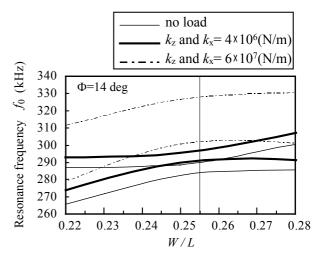
Fig.4 Resonance frequency correlated with the width-to-length ratio *W/L* depended on the load of springs.
