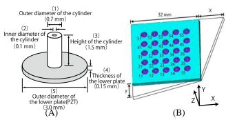
Fig. 3 Analysis model of (A) the stator and (B) the array. About the stator model, the round of the PZT is perfectly in the fixed condition.
