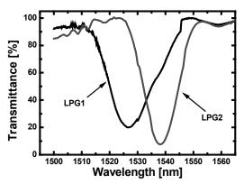
Fig.4. Transmission spectra of sensing LPGs.
