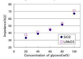
Fig. 2 Impedance spectrum of IDE sensors on SiO<sub>2</sub> and LiNbO<sub>3</sub>
