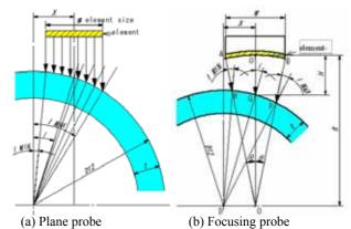
Fig. 1 Oblique incidence to pipes. by NAUT
