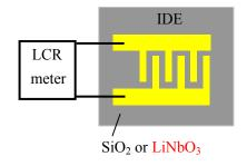
Fig. 1 IDE sensor system.
