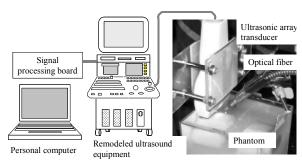
Fig.1 Experimental set-up
