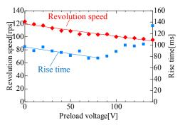
Fig.4 Revolution speed and rise time as a function of preload voltage.
