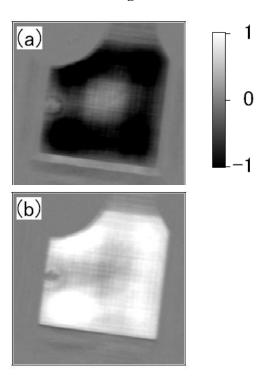
Fig. 3 Experimental time-resolved surface vibration images for a 220  $\mu$ m × 220  $\mu$ m region of the FBAR. (a) and (b) correspond to a time difference of 6790 ps.
