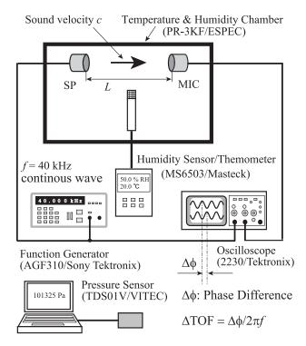
Fig. 1 Schematic of experiment.
