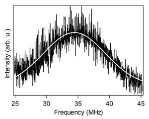
Fig. 2 Brillouin peak in PMMA observed with the millisecond Brillouin spectroscopy. The white solid line is the best-fitted Gaussian curve. The sampling rate and measurement time are 500 MS/s and 10 ms, respectively. The scattering wavenumber is  $k = 8.1 \times 10^4$  m<sup>-1</sup>.
