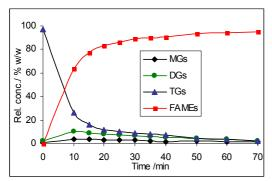
Fig.2 Time profile of reactant and products for transesterification reaction of canola oil to FAMEs with molar ratio of oil to methanol 1:5, KOH 0.7%
