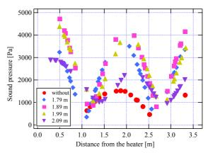
Fig. 4 Distribution of sound pressure in loop-tube.
