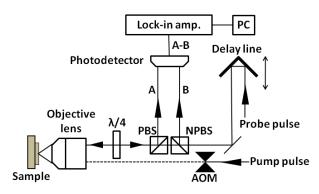
Fig. 2 Experimental setup for generation and detection of nanopillar vibrations. AOM: acousto-optic modulator, PBS: polarizing beam splitter, NPBS: non-polarizing beam splitter, PC: personal computer,  $\lambda/4$ : quarter-wave plate.
