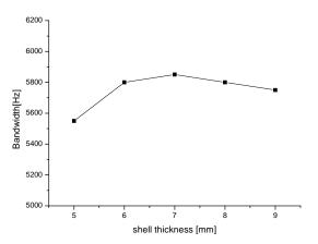
Fig. 2 Variation of performance in relation to shell thickness.
