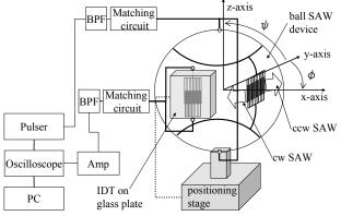
Fig. 2 Schematic of measurement system
