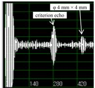
Fig. 5 Example of detecting 4 mm × 4 mm deep flat bottom hole
