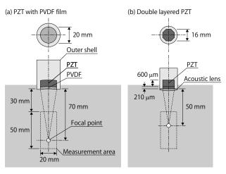
Fig. 1 Configuration of the proposed transducers.
