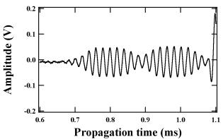
Fig. 4 Time domain signal without the reflector. The first wave packet indicates the signal of the left side defect which had already introduced in the previous experiment with the reflector.
