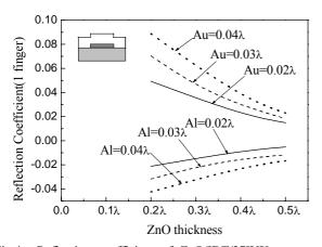
Fig.4 Reflection coefficient of ZnO/IDT/27°YX quartz as function of ZnO thickness at Au and Al thickness of 0.2, 0.3, 0.4 .(Metalization ratio)
