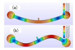
Fig. 3 The bending modes of the vibrator with counterweight
