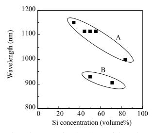
Fig. 3 Si concentration dependence of absorption band edge wavelength of amorphous Si.
