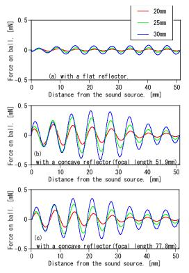
Fig. 2. Calculated force on steel ball along the sound beam axis.
