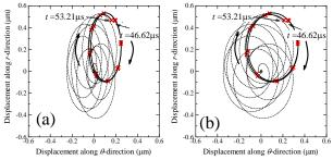
Fig. 2 Analytical result of surface particle motion for low frequencies at (a) outer surface and (b) inner surface.
