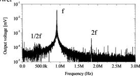
Fig. 5 FFT analysis result of a hydrophone probe output (12ppm, 30W)
