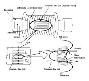
Fig. 1 Configuration and mechanism of the magnetostrictive EMAT for generating and receiving the axial shear wave.
