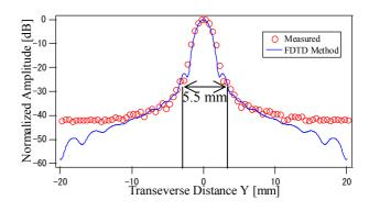
Fig.4 Measured and Simulated Acoustic Fields along Axis Y
