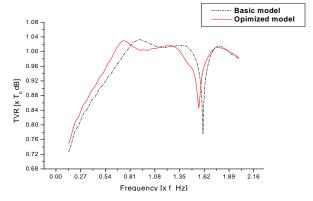
Fig. 3 TVR spectrum of the basic and optimized models
