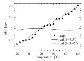
Fig.3 Comparing measurement and theoretical analyses of frequency-temperature characteristics
