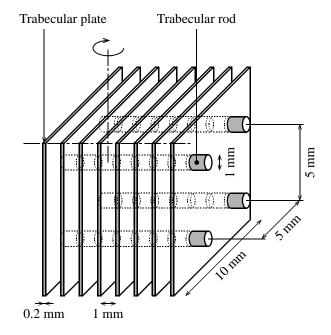
Fig. 1 Geometry of a stratified trabecular phantom.
