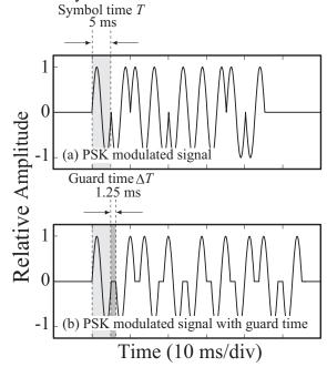
**Fig.2** PSK modulated signal and PSK modulated signal with GT to reduce the affection of impulse.
