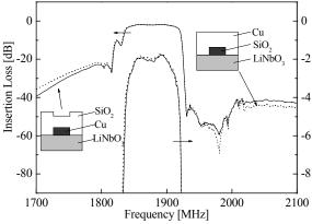
Fig5. Tx filter response of flattened structure and conex structure
