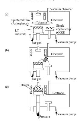
Fig. 5. Fabrication process by the contactepitaxy
