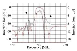
Fig. 6: Frequency characteristic of RF filter with flattened SiO<sub>2</sub> film/high density metal electrode/36°-48°Y·X-LiTaO<sub>3</sub> substrate. (broken line: Phase inverse design, solid line: Normal design)
