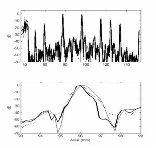
Fig. 4 Axial lines through the center of the quality assurance phantom. Thick: The QF1. Thin: The QF2. Dash: The QF3.
