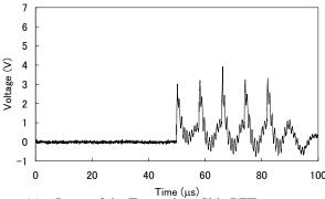
(a) Input of the Transmitter Side PZT.
