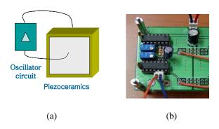
Fig. 2 Oscillator sensor; (a) schematic structure of the sensor (b) photograph of the oscillator circuit
