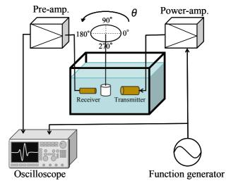
Fig. 2 Ultrasound measurement system.
