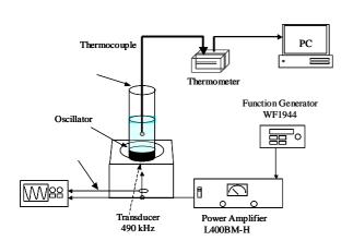
Fig. 1 Experimental set-up for power measurements.
