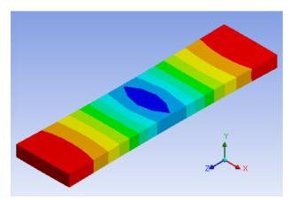
Fig. 2 Longitudinal vibration mode of the ultrasonic motor.
