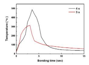
Fig. 1 Temperature rise during 3 and 4 s of ultrasonic bonding
