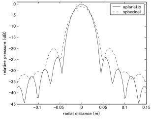
Fig. 2 Beam patterns of normal incidence.
