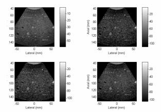
Fig. 3 Top Left: B-mode image of a quality assurance phantom. The images from the QF1, QF2, and QF3 are shown at Top Right, Bottom Left and Bottom Right, respectively.
