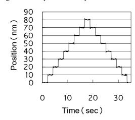
Fig. 4 Step positioning of 10 nm.
