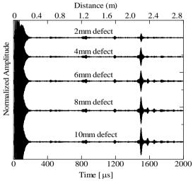
Fig. 6 Normalized amplitude with propagation time for different defect order.
