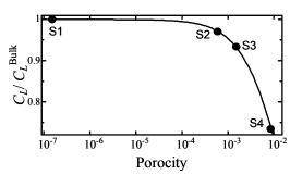
Fig. 3 Relationship between the measured and calculated elastic constants  $C_L$  for the defects with the aspect ratio 1/100.
