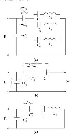
Fig. 1 (a) Lumped-parameter equivalent circuit. The switch  $SW_{DP}$  is opened for L-effect and shorted for T-effect. (b) In the quasi-static situation (with mechanical terminal). (c) When the nth mode is observed.
