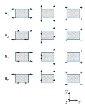
**Fig. 2.** Symmetry-adopted basis functions belonging to the irreducible representations of  $C_{2\nu}$ . Arrows and  $\pm$  show the phonon displacements at the corners.
