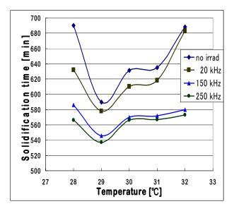
Fig.2. Solidification time dependent on temperature in the case of ultrasonic irradiation
