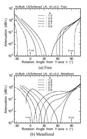
Fig. 3 Calculated attenuation.
