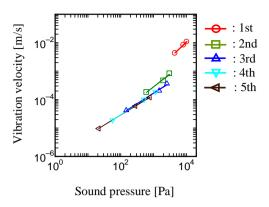
Fig. 3 Relationship between sound pressure and vibration velocity of sample MS20 at the converging point.
