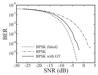
**Fig.4** BER performance of BPSK modulated signal and BPSK modulated signal with GT observed in performance evaluation system.
