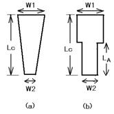
Fig.4 Horn type longitudinal bar resonator.
