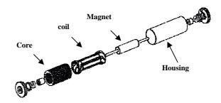
Fig. 2 The construction of the tested motor
