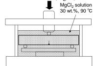
Fig. 2. Experimental setup for SCC formation.
