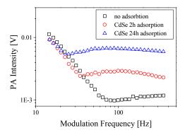
Figure 2 Modulation frequency dependence of PA signal intensity of NSi adsorbed with CdSe QDs.
