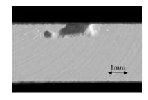
(b) xz-plane view from y-direction fig. 2 Photograph of compound weld defect
