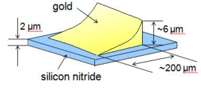
Fig. 1 Schematic diagram of a gold wedge on a silicon nitride membrane.
