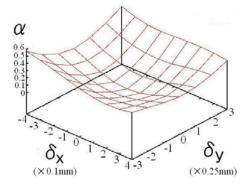
Fig. 3 Typical distribution  $\alpha(\delta_x, \delta_y)$  of constrained least square errors in Fig. 2 shows the minimum at the original positions of successive two echo frames.
