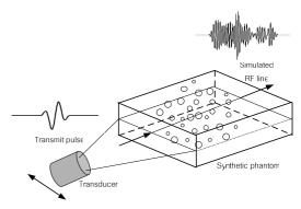
Fig. 2 A diagram showing the generation of an RF line from a nonlinear pulse-echo system (NPS).
