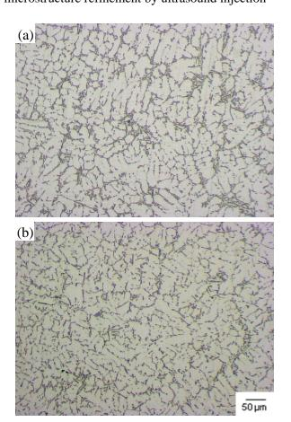
Fig. 2 Microstructure of A356 alloy; (a) without and (b) with ultrasound injection for 10 min.
