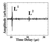
Fig.2 Ultrasonic performance of IUT in Fig.1 at 800°C
