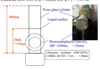
Fig. 1 Experimental setup for measurement of sonoluminescence
