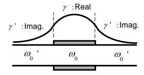
Fig. 1(b) Displacement distribution for trapped-energy mode.
