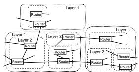
Fig.1 Two-layer photonic network.
