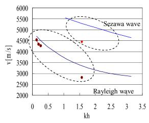
Fig.1 Difference of measured and simulated SAW velocity vs *kh*.
