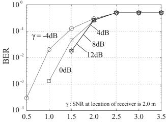
Location of receiver and noise source Fig. 5 BER performance with transmitters-A and -B.
