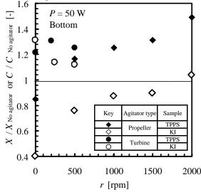
Fig.4 Effect of revolution rate on ratio of TPPS decomposition conversion or I<sub>3</sub>- concentration for single irradiation from bottom with agitator
