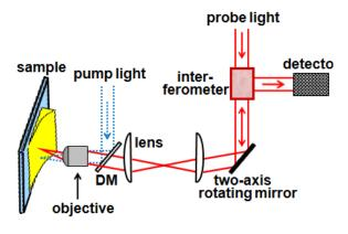
Fig. 2 Measurement setup DM: dichroic mirror
