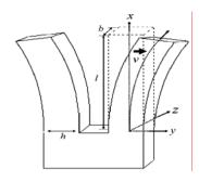
Fig.1 Configuration of Quartz Crystal Tuning Fork
