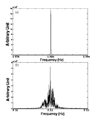
Fig. 3 FFT of the waves from quartz crystal (a) in air (b) in water
