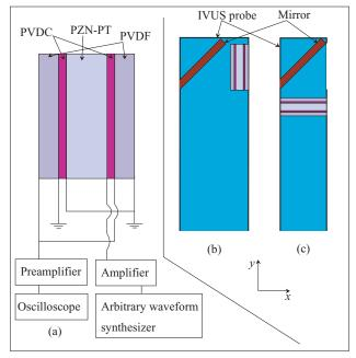
Fig.1 (a) A diagram of inline transmitter/receiver system with canceling function, and proposed structures; (b) type-1 and (c) type-2
