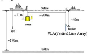
Fig.1 Schematic diagram of experimental configuration.
