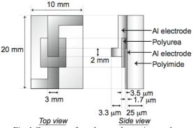
Fig. 1 Geometry of a polyurea ultrasonic transducer.
