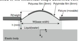
Fig. 3 Geometry of the surface acoustic wave velocity measurement.
