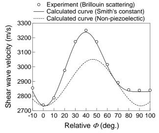
Fig. 4 In-plane anisotropy of shear horizontal wave velocity of the ZnO single crystal measured by Brillouin scattering.
