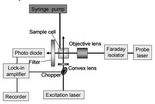
**Figure 1.** Schematic diagram of photothermal lens detection system
