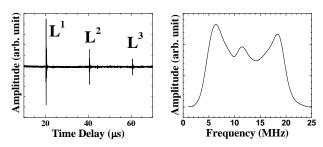
Fig. 6 Ultrasonic performance of BIT/PZT IUT fabricated onto the surface of a thixomolding mold.
