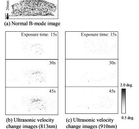
Fig.3 Normal B-mode image and ultrasonic velocity images of the phantom
