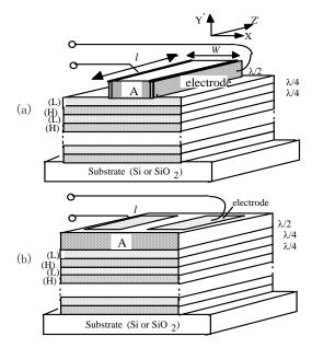
Fig. 1 Shear mode SMR by parallel field excitation. A: Rotated Y-cut LiTaO<sub>3</sub> film.
