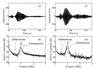
Fig. 3. (a) The received waveform and (b) its spectrum in no-crack area. (c) The waveform and (d) its spectrum in closed crack area.
