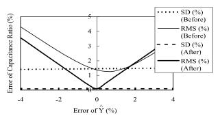
Fig. 4 Dependence of the root-mean-square error (RMS) and standard deviation of error (SD) of the estimated capacitance ratio on the error of inferred  $\hat{Y}$ , before and after the correction of  $g_n$ .
