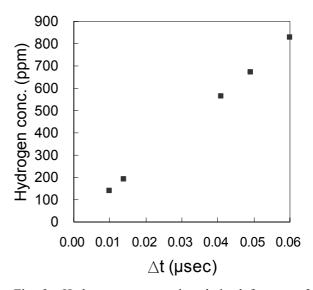
Fig. 3 Hydrogen concentration derived form eq. 2 with the measured  $\Delta t$ : the traveling time difference between the air and the hydrogen contained air.
