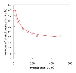
Fig. 3. Sonochemical degradation of phenol as a function of cyclohexanol concentration.
