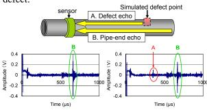
A. Non-defect signal B. Defect signal (15%) Fig.9 Example of received ultrasonic waveforms
