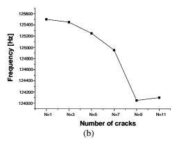
Fig. 1 Resonant frequency of the PZT sensor vs. (a) crack length and (b) crack number
