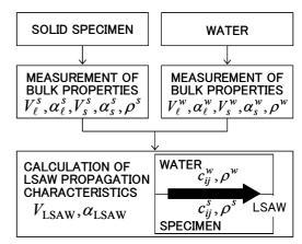
New concept of theoretical analysis of LSAW propagation characteristics.
