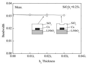
Fig3. Bandwidth as a function of h<sub>2</sub> thickness
