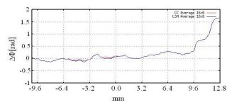
Fig. 2 The comparison of local phase change evaluations by conventional cross-correlation method and constrained least square method within a frame interval (1 ms).
