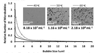
Fig. 2: Effect of solution temperature on the concentration and size distribution of BSA microbubbles produced from 10 second sonication.
