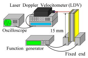
Fig.4 Vibration velocity measurement system of bimorph type vibrator with hydrothermally synthesized PZT polycrystalline film
