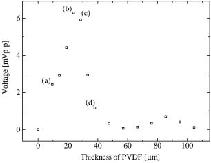
Fig. 2 : Voltages of echo signals received by PVDF film with various thicknesses.
