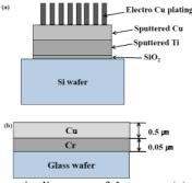
Fig. 1 Schematic diagrams of the upper (a) and lower (b) substrates used in this study.
