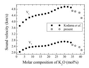
Fig. 3 The composition dependence of sound velocity.
