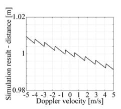
Figure 3: The distance measured from the Doppler-shifted TOF
