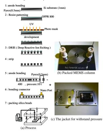
Fig.2 Fabrication of micro separation column that uses MEMS technology
