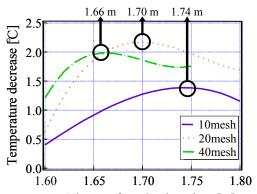
Distance from loudspeaker [m] Fig. 3 Temperature decrease as a function of the stack distance from the loudspeaker (three-dimensional approximated curve).
