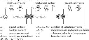
**Fig. 1** Equivalent circuit of loudspeaker.
