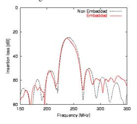
Fig.4 Frequency response of the filter using embedded and non-embedded IDTs
