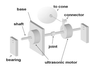
Fig5 Dual motor model
