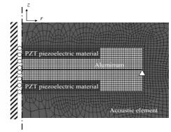
Fig. 2 Transducer simplified model for FEM analysis.
