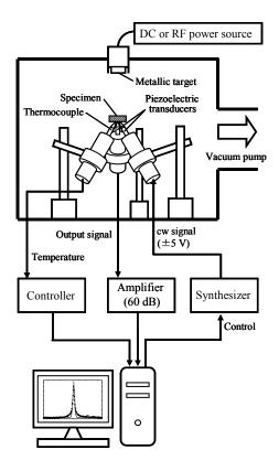
Fig. 1 Setup of sputtering/RUS monitoring system.
