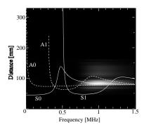
Fig. 4. Dispersion curves of group velocity of Lamb wave in glass and result of wavelet transform of received waveform.
