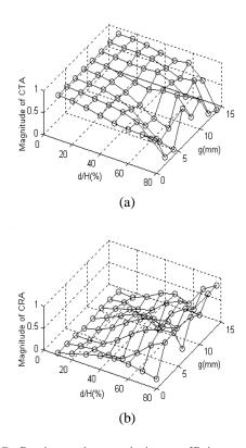
Fig. 3 Reflection and transmission coefficients when  $A_0$  mode wave is incident; (a) transmission coefficient of  $A_0$ , (b) reflection coefficient of  $A_0$
