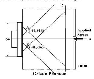
Fig. 1 Experimental setup for external stress input and alternate irradiations by two virtual point sources A and B across a 1 % gelatin phantom including 1 % fine starch powder.
