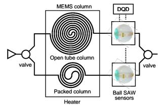
Fig.1 The concept of Dual column ball SAW GC
