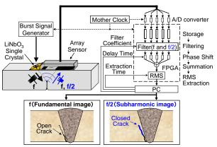
Fig. 1. Experimental configuration of SPACE.
