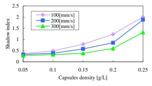
Fig.4 Shadow index versus capsules density.
