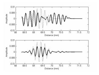
Fig. 4 Quadratic outputs from the algorithm without (Top) and with (Bottom) TSVD regularization when the number of input sequences is decreased from 64 to 16.
