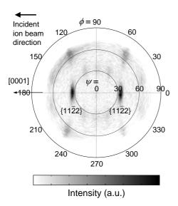
Fig. 3 (1122) pole figure of (1120) textured AlN film (sample A). The arrows indicate the [0001] direction in the substrate plane and the incident ion beam direction.
