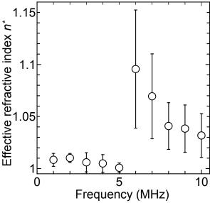
Fig. 3 Measured effective refractive index for small amplitude focused ultrasound (Light wavelength = 633 nm, Water temperature = 22.0°C).
