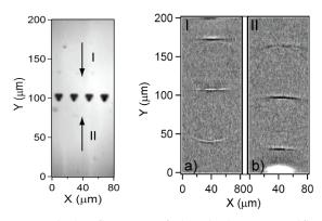
Fig. 3 Optical reflectance of the single row rectifier structure: I and II indicate the direction of incident SAW's. a) and b) are the phase difference images at delay time 0.51 ns for cases I and II, respectively. The bright spot b) is the pump position.
