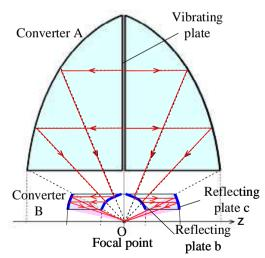
Fig. 2 Arrangement of two converters and converging of the ultrasonic waves.
