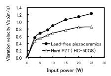
Fig.3. Variation of the vibration velocity of BLT (Bolt-clamp Langevin Transducer) with the input power.
