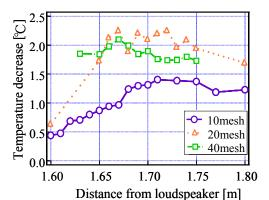
Fig. 2 Temperature decrease as a function of the stack distance from the loudspeaker.
