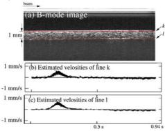
Fig. 2 (a) B-mode image of the silicone rubber.(b) and (c) Estimated velocities at lines k and l obtained at 127 ultrasonic beam positions.
