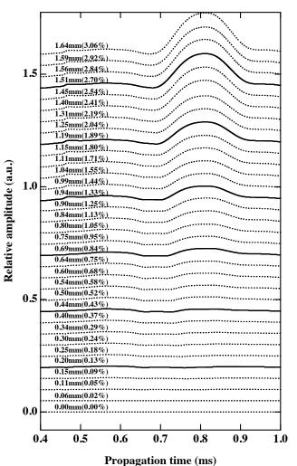
Fig. 5 Enveloped signals for different depth defects.
