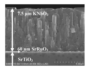
Fig.2 Cross-sectional SEM photograph of 7.5 μm-thick epitaxial KNbO<sub>3</sub> film.
