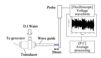
Fig. 3 Schematic diagram of sound pressure measurement using hydrophone probe
