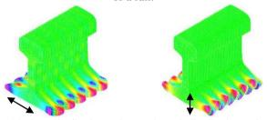
(a) horizontally vibrating mode (b) vertically vibrating mode Fig.2 Visualization of the vibrating modes corresponding to the arrow positions in Fig.1 (a) and (b).
