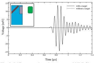
Fig. 2: Difference voltage between two PVDF films using Type-1 structure with a target stainless steel (solid line) and without a target one (broken line)
