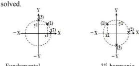
respectively. In Fig.(a) assuming the phase of output (2) to be  $0^{\circ}$ , output (3) has  $90^{\circ}$  phase due to  $\lambda 0/4$ -length difference between two delay lines. Output (1) is located in between as shown in the figure and moves along the circle depending on
