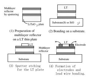
Fig. 5 Fabrication process of the SMR.
