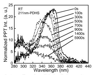
Fig. 2 Effect of UV-light irradiation on the PPT spectrum of 211-nm-thickness sample
