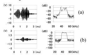
Fig.3 (a): Adaptive signal; (b): Reference receiving signal.
