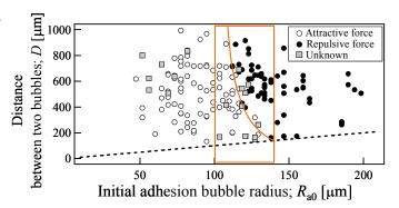
Fig.3 Direction of interactive force in  $R_{a0}$ - D plane.
