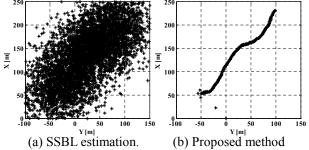
Fig. 1 Simulation result of AUV positioning. The true track is well tracked in the right figure.
