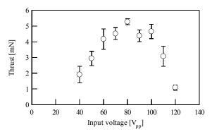
Fig. 4 The stage thrust vs. the input voltages to the channels 1 and 3.
