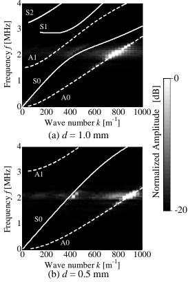
Fig.5 *k-f* image lapped dispersion curves.
