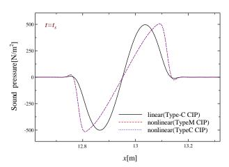
Fig. 2 Sound pressure distribution at  $t_s$
