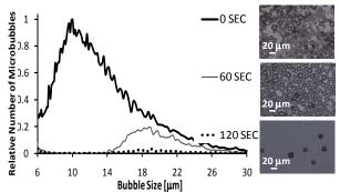
Fig. 5: Effect of sonication time on size distribution of microbubbles (727 kHz with an applied power of 40 W).
