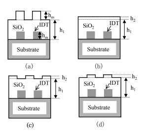
Fig1. SiO<sub>2</sub>/Cu-electrode/LiNbO<sub>3</sub> structure
