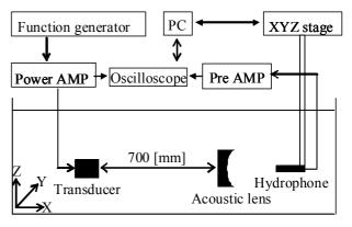
Fig. 1 Block diagram of measurement
