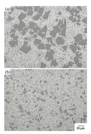
Fig. 3 Microstructure of A390 alloy; (a) without and (b) with ultrasound injection for 10 min.
