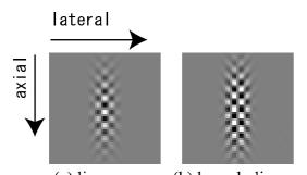
(a) linear scan (b) hyperbolic scan Fig. 1 Lateral modulated RF at depth 50mm, *x*=0mm
