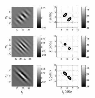
Fig. 2 Left: Coefficients of the QF. Right: The magnitude of 2D frequency response of the QF.
