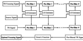
Fig.3 Signal-flow graph of ILS-PF method
