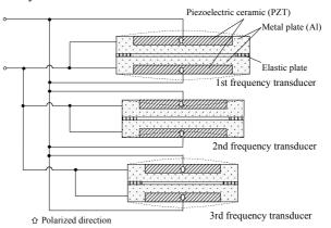
Fig. 3 Chart of connecting wires of low frequency and wideband array composed of disk bender transducers having differential connections.
