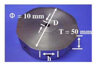
Fig.4 Vibrating compaction die.
