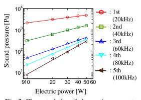
Fig. 2 Characteristics of ultrasonic waves at the converging point.
