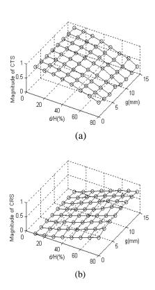
Fig. 2 Reflection and transmission coefficients when an  $S_0$  mode wave is incident; d/H (%) is the ratio of crack height/plate thickness: (a) transmission coefficient of  $S_0$ , (b) reflection coefficient of  $S_0$
