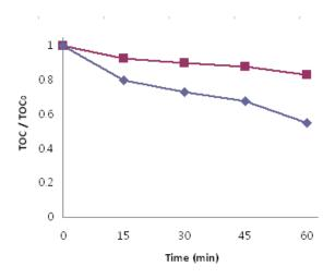
**Fig. 3** The mineralization of C.I. Reactive Black 5 (■ : Fenton process, ◆ : Sonochemical + Fenton process), reaction condition -  $H_2O_2 = 120 \text{mgL}^{-1}$ ;  $H_2O_2$ :FeSO<sub>4</sub> = 1:4; [dye]<sub>0</sub> =  $100 \text{mgL}^{-1}$ ; frequency = 35 kHz; power = 400 W
