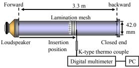
Fig. 1 Block diagram of measurement system.
