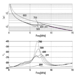
Fig.2 electric impedance after 120V driving. Numbers in the graph indicate cycle numbers of driving burst waves.
