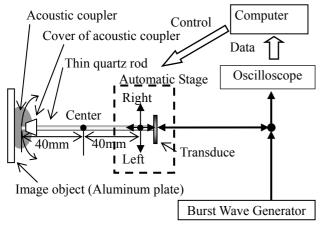
Fig. 3. Schematic diagram of measurement.
