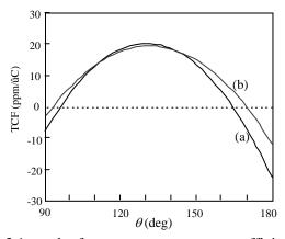
Fig. 3 1st order frequency temperature coefficient. (a) Rotated Y-cut LiTaO<sub>3</sub> shear wave resonator.
