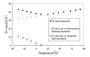
Fig.3 Temperature-CI value characteristics
