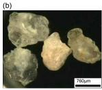
Fig. 1 Photograph Image: (a) Shredded rubber; (b) Jumunjin 20/30 sand.
