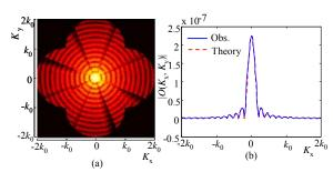
**Fig.3** Calculated object function: (a) gray scale image of  $\log(|O(K_x,K_y)|)$  on Fourier plane and (b) cross sectional profile of  $|O(K_x,K_y)|$  on  $K_x$  axis (solid line show the result from the scattered data, dotted line from the theory).
