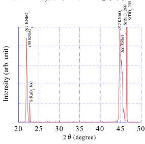
Fig.1 XRD pattern of KNbO<sub>3</sub> film grown on (100)SrRuO<sub>3</sub>//SrTiO<sub>3</sub> substrate using hydrothermal method.
