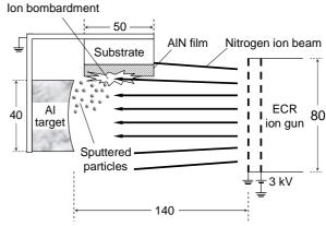
Fig. 1 Ion beam sputtering deposition system with single ion gun.
