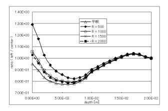
Fig. 3 Strain ratio using a concave compression board
