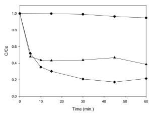
**Fig. 2.** Comparison of individual and combined schemes for tannins degradation (0.100 L,  $25 \pm 3^{\circ}$ c,  $[C_{76}H_{52}O_{46}] = 0.3$  mM); •, US only (170 kHz, 400 W); •,  $O_3$  only (1 g L<sup>-1</sup>); •, US +  $O_3$ )
