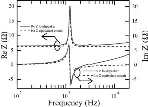
Fig.3 Impedances of an actual loudspeaker and its equivalent circuit.
