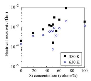
Fig. 1 Si concentration dependence of electrical resistivity at second annealing cycle.
