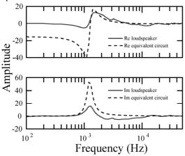
Fig. 5 Frequency response of loudspeaker and equivalent circuit.
