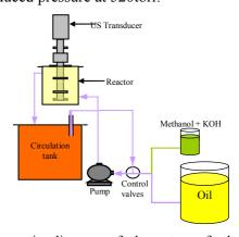
Fig.1 Schematic diagram of the setup of ultrasonic circulation process for BDF production
