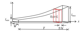
Fig. 1. Calculation model for piezoelectric vibrator with exponentially tapered thickness.
