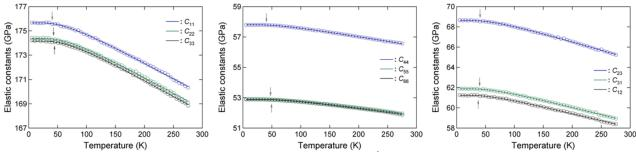
Figure 1. Temperature dependence of elastic constants  $C_{ij}(T)$  of C12A7:  $O^{2-}$  single crystal determined by EMAR. Arrows show Einstein temperatures estimated from Varshni's equation.<sup>6)</sup>
