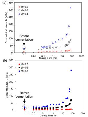
Fig. 5 Modulus change during cementation: (a) constraint modulus; (b) shear modulus.
