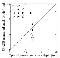
Fig. 6. Relationship between optically- and SPACE-measured crack depths of the SCC.
