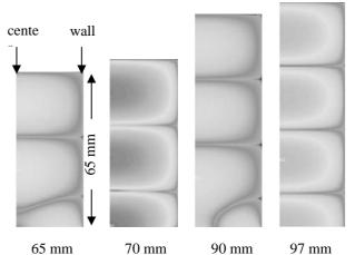
Fig. 3 Calculated spatial distribution of the pressure amplitude. The liquid height of 80 mm and 97 mm are better stable on sound pressure field.
