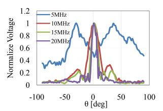
Fig. 3 Transmission directivity of miniature ultrasound probe
