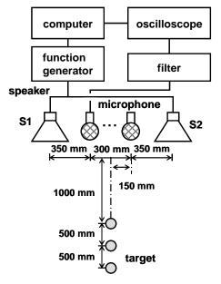
Fig. 1 Measurement system.
