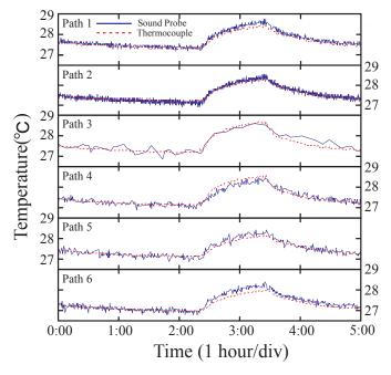
Fig.3 Temperature transitions along six acoustic paths.
