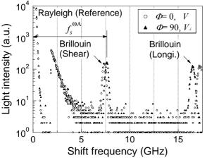
Fig. 3 Typical Brillouin spectra obtained from the ZnO single crystal. Open circle and solid triangle show the spectra measured at  $\Phi = 0^{\circ}(V)$ , respectively.
