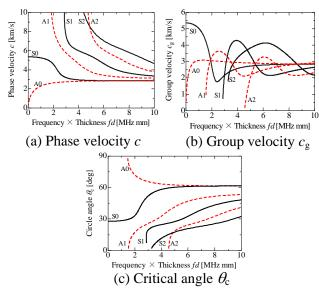
Fig.1 Dispersion curves of Lamb wave in aluminum.
