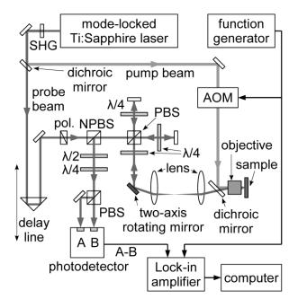
Fig. 1. Schematic diagram of the imaging system. SHG: second harmonic generation crystal, AOM: acousto-optical modulator, pol.: polarizer, NPBS: non-polarizing beam splitter, PBS: polarizing beam splitter,  $\lambda$ 4: quarter-wave retarder, and  $\lambda$ 2: half-wave retarder.
