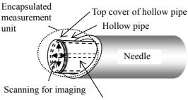
Thin rod (as a transmission line and sensor)
