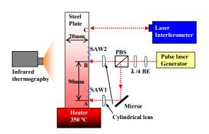
Fig. 2 Schematic of the laser ultrasonic system used for measuring SAWs on a steel plate being heated.
