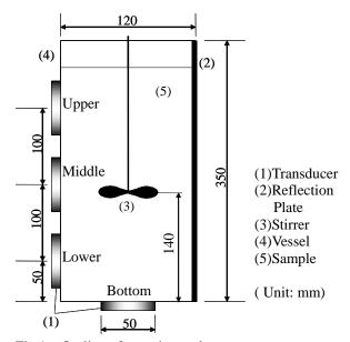
Fig.1 Outline of experimental apparatus
