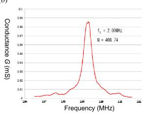
Fig. 2 Frequency response of admittance (a) and Conductance (b) for the vibrator.
