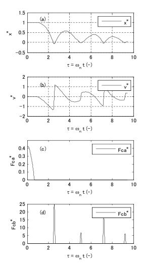
Fig.2 Time history of non-dimensional variables of contact. (a) Displacement  $x^* = x/G$ . (b) Velocity  $v^* = v/(\omega_n G)$ . (c) Contact force  $F_{ca}^* = F_{ca}/(kG)$ . (d) Contact force  $F_{cb}^* = F_{cb}/(kG)$ .
