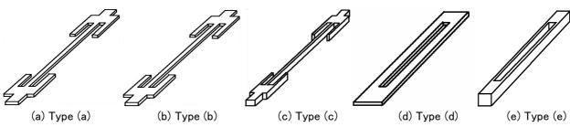
Fig. 1 Structures of frequency-change-type force sensor.
