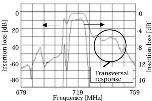
Fig. 1 Frequency characteristic of RF filter with conventional Al/36°-48°Y·X-LiTaO<sub>3</sub> substrate.
