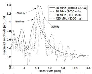
Fig. 4 Frequency characteristics of V(W) curve (h=0.5 mm, Frequency=30, 60, 120MHz,  $v_{LSAW}$ =3000 m/s).
