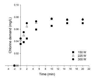
**Fig. 4** Chlorine demand for different powers in the condition of 2 min irradiation
