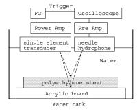
Fig. 2 Schema of the experiment.
