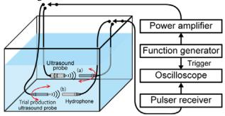
Fig. 1 Directive measurement system
