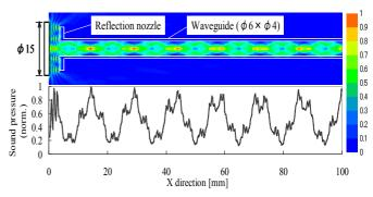
Fig.2 Propagation in the waveguide predicted by Cellular Automata
