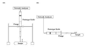
Fig. 2 Experimental setup. (a) End of tip contacts. (b) Side of tip contacts.
