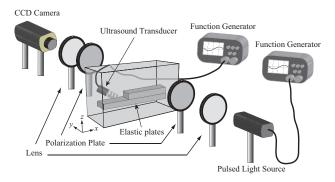
Fig. 1 Visualization systems of sound waves.
