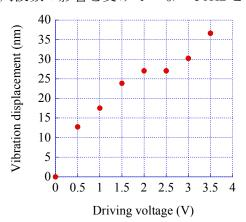
Fig.4 Relationship between vibration displacement and applied voltage at 50 Hz.
