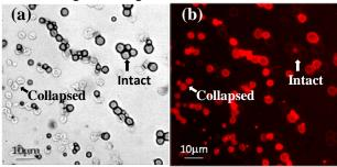
Fig. 4: (a) Light illumination showing microbubbles that has been dried on a glass plate. (b) Same sample as (a) but showing fluorescence emission from microbubbles that were not cross-linked by glutaraldehyde.
