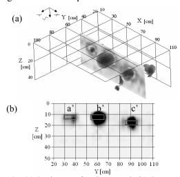
Fig. 4 (a) 3D image of underground. (b) Cross section materials and buried depth Z[m] are a': resin model, 10 cm. b': hollow container, 10 cm. c': hollow container, 15 cm
