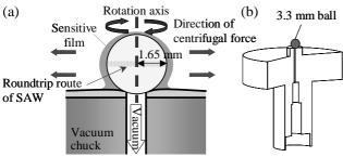
Fig.1 Schematic diagram of conventional spin coating method (a) and cross-section drawing of the vacuum chuck (b)
