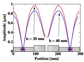
Fig. 5 Vibration distribution in the radial direction.
