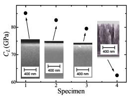
Fig. 2 Elastic constants  $C_L$  and cross-section microstructures of a-SiO<sub>2</sub> films.
