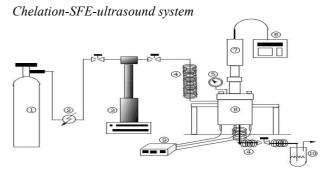
①  $CO_2$  cylinder ② condenser ③ syringe pump ④ heating coil ⑤ pressure gauge ⑥ ultrasonic power generator ⑦ ultrasonic transducer ⑧ high-pressure extractor ⑨ temperature controller ⑩ separator
