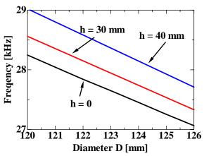
Fig. 6 Relationship between the diameter of die and the resonance frequency for the radial mode.
