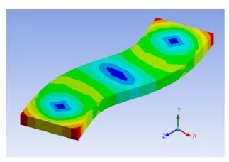
Fig. 3 Bending vibration mode of the ultrasonic motor.
