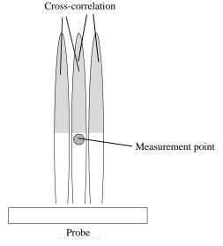
Fig. 1 Cross-correlation between RF signals of adjacent scan lines for calculi detection.
