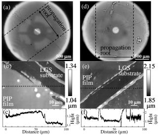
Fig.3 Optical microscope images (a),(d) and topographies (b),(e) of the PIP films coated by conventional method and off-axis method, respectively. (c),(f) Profiles along the dashed lines in (b),(e), respectively.
