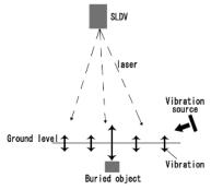
Fig.1 Fundamental concept of exploration method using SLDV
