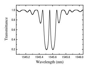
Fig. 2 Transmittance spectrum of FPI with FBG
