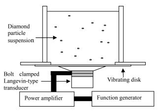
Fig. 1 Acoustic dispersion system for improvement of disaggregation and surface modification of nanometer-sized diamond particles
