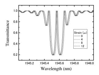
Fig. 5 Strain dependence of transmittance spectrum of FBG-FPI.
