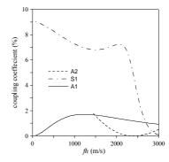
Fig.6 Coupling coefficient for metalized surface calculated by the acoustic velocity difference method.
