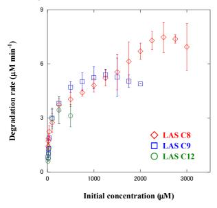
**Fig. 2** Relationship between the concentration of LASs and their initial sonochemical degradation rate.
