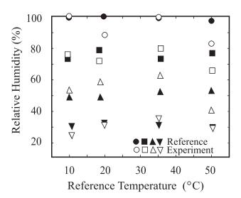
Fig. 2 Relative humidity measured in the chamber at various temperatures.
