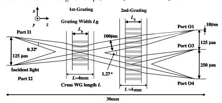
Fig. 1 Analytical model of 3-output-ports type tandem AOFS.
