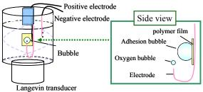
Fig.1 Experimental cell.
