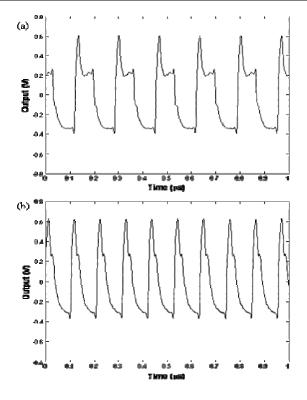
Fig. 2 The waveform of the signals from quartz crystal (a) in air, (b) in water
