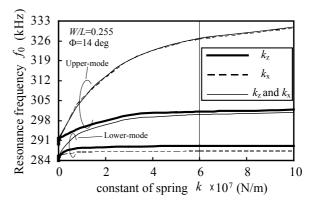
Fig.2 Analysis result of the resonance frequency correlated with spring constant *k* of loads.
