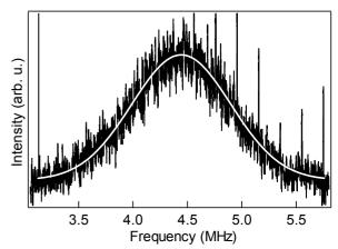
Fig. 4 Brillouin peak observed with the millisecond Brillouin spectroscopy in air. The white solid line is the best-fitted Gaussian curve. The sampling rate and measurement time are 250 MS/s and 200 ms, respectively. The scattering wavenumber is  $k = 8.1 \times 10^4$  m<sup>-1</sup>.
