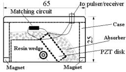
Fig. 3 Transducer for a rail bottom edges.
