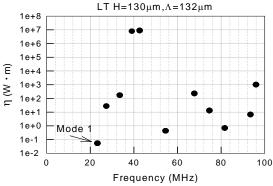
Fig.3 Analytical result of Lamb wave power in each mode for polarized wave rotation.
