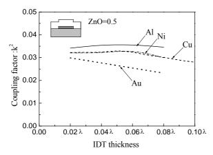
Fig.3 Coupling factor of ZnO/ various  $IDT/27^{\circ}YX$  quartz as function of IDT thickness at ZnO thickness of 0.5
