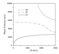
Fig. 2 Phase velocity dispersion of the first three Lamb modes with free surface.
