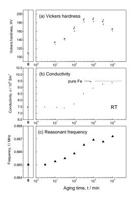
Fig. 2 Aging time dependence of the Vickers hardness, conductivity and typical resonant frequency.
