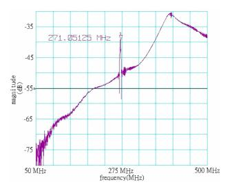
Fig. 2. The measured frequency response of the SAW filter for  $Al_2O_3$  (1.45  $\mu$  m thick)/ST-cut quartz substrate with electrode width of 3  $\mu$ m.
