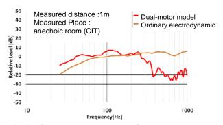
Fig 6 Output sound pressure frequency response
