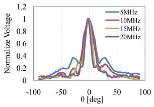
Fig. 4 Receiving directivity of miniature ultrasound probe
