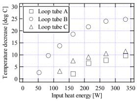
Fig.2 Temperature decrease at the cooling point measured for various input heat energy.
