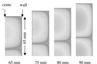
Fig. 1 Calculated spatial distribution of the pressure amplitude. The liquid height of 80 mm is the most stable on sound pressure field.
