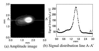
Fig. 5 PA amplitude image and signal distribution for the specimen with compound weld defect (modulation frequencies: 270Hz)
