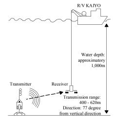
Fig.1 Geometry of the sea experiment.
