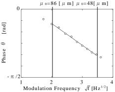
Fig. 5 Relation between  $\theta$  and  $\sqrt{f}$  in the PET film
