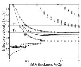
Fig. 4 Variation of the effective velocities of acoustic waves with  $h_2/2p$  (Controlled: Cu  $h_1=h_3=0.2$  p)
