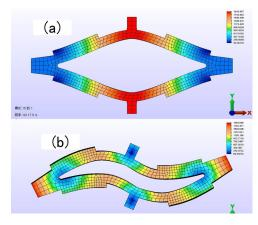
Fig. 5 The bending modes of the vibrator with diamond hollow structure
