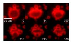
Fig. 3: Selecterd frames from a frame rate of 30f/s documenting the collapse of a 10  $\mu$ m bubble due to the diffusion of gas in a degassed medium.
