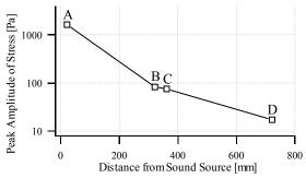
Figure 5: The changes of peak amplitudes from point A to D.
