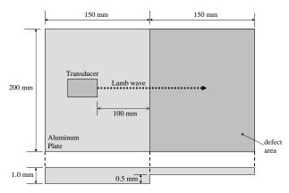
Fig.3 Aluminum plate used in this experiment.
