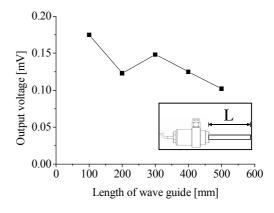
Fig. 5 Dependence on the length of waveguide
