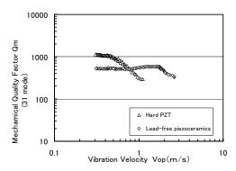
Fig.2. Variation of the mechanical quality factor  $Q_m$  with the vibration velocity.
