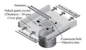
Fig. 1 Schematic illustration of developed TIRFM-QCM sensor cell. One antenna oscillates the quartz oscillator with constant resonance frequency, and the other antenna receives the resonance frequency through electromagnetic waves while solution flows. White part is visible and black part is invisible by TIRFM, however quantitative change of the mass on the all over the oscillator surface can be detected by the WE-QCM.
