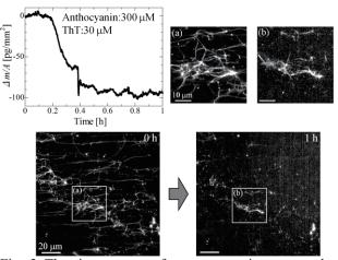
Fig. 2 The time course of mass per unit area on the surface measured by WE-QCM and fluorescence images at same point by TIRFM in dissociation process as flowing poly-phenol anthocyanins solution.
