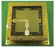
Fig. 5 Two-axis sensor of trial production.
