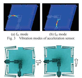
(a)  $\alpha$  to the x axis direction (b)  $\alpha$  to the y axis direction Fig. 4 Analyzed motion of mass applying acceleration.
