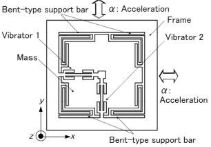
Fig. 2 Structure of two-axis acceleration sensor.
