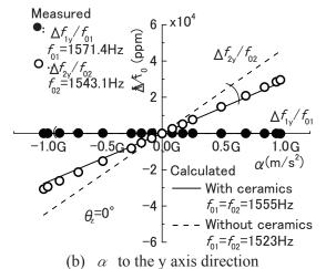
Characteristics of sensor of trial production. Fig. 6
