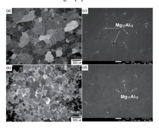
Fig. 2. Macro((a) and (b)) and grain boundary ((c) and (d)) structure of AZ31 alloy cast without (((a) and (c)) and with NEUMT((b) and (d))
